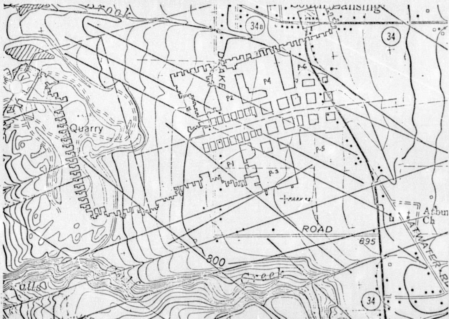
Figure 7. Roof conditions and surface lineaments in "No.6" salt seam.
