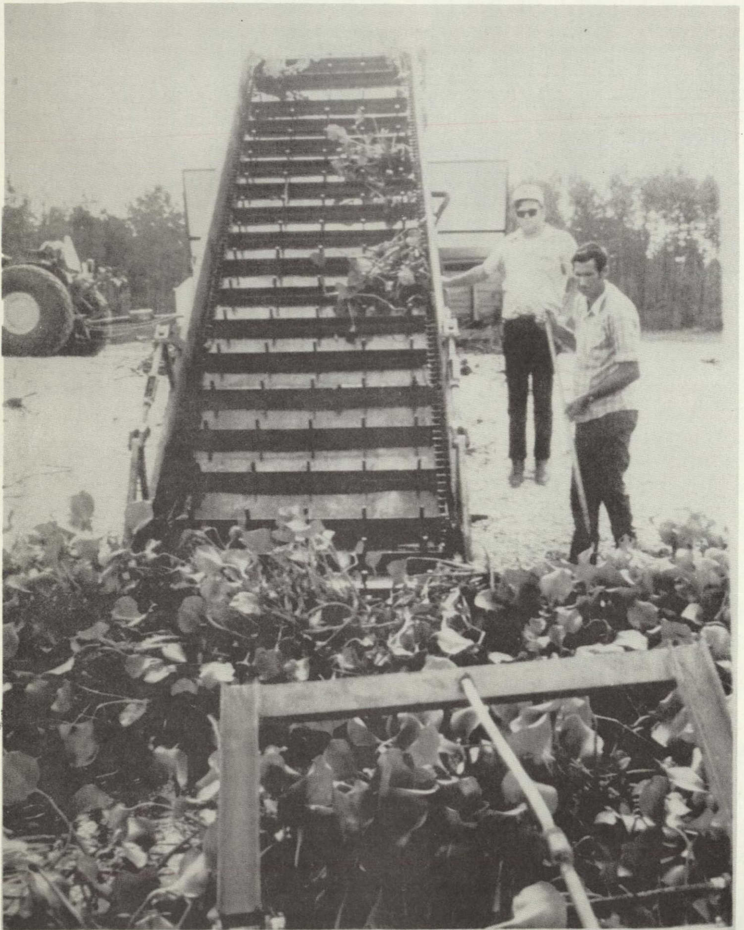
Figure 4. Single conveyor harvester
