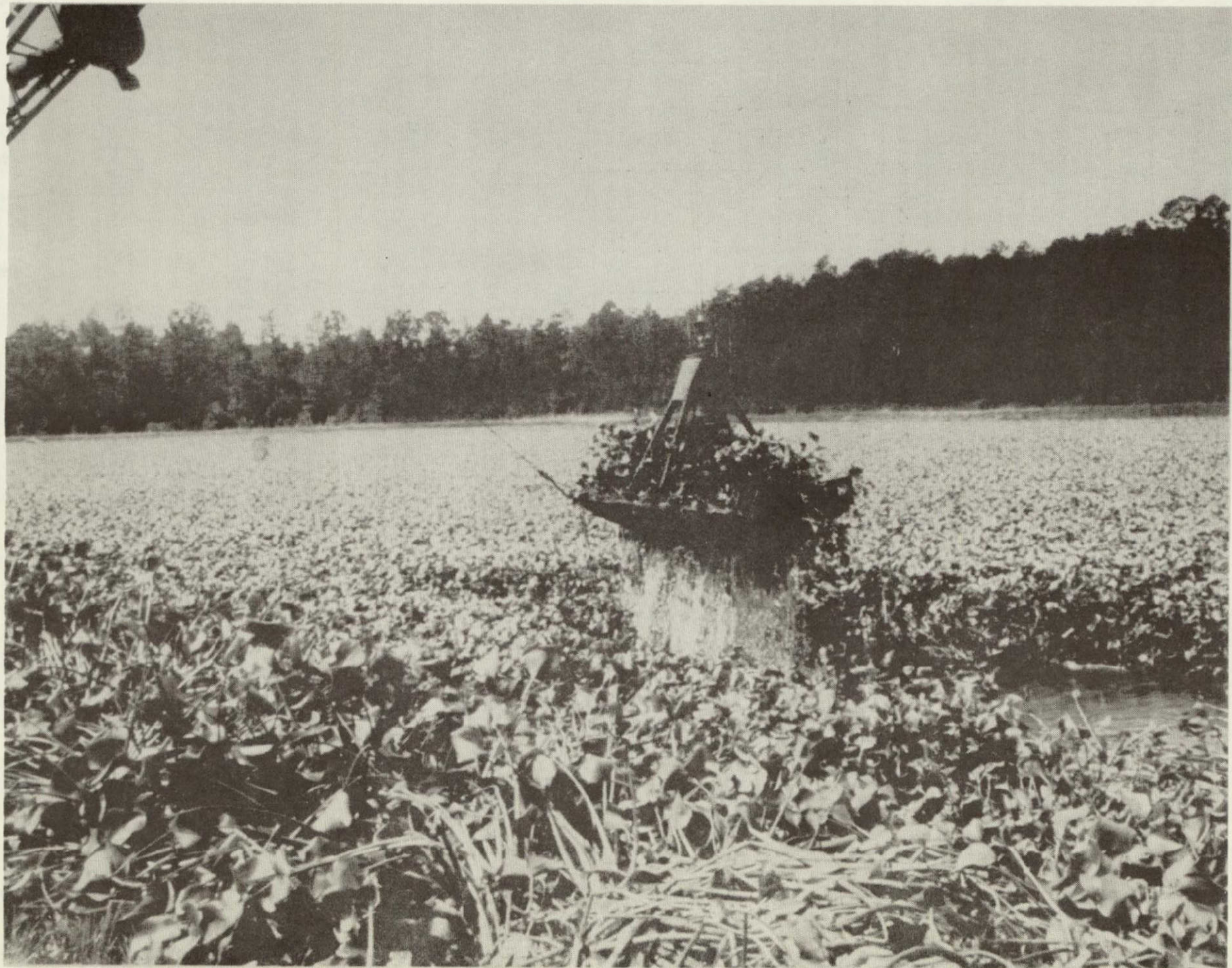
Figure 5. Modified clam-shell bucket
