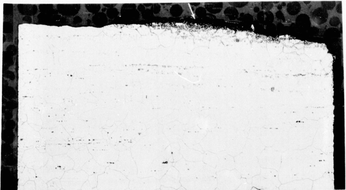
Figure 52. Cross-section of Blade from Test 17 Showing Decomposition of the Grain Structure (Mag: 100x)
