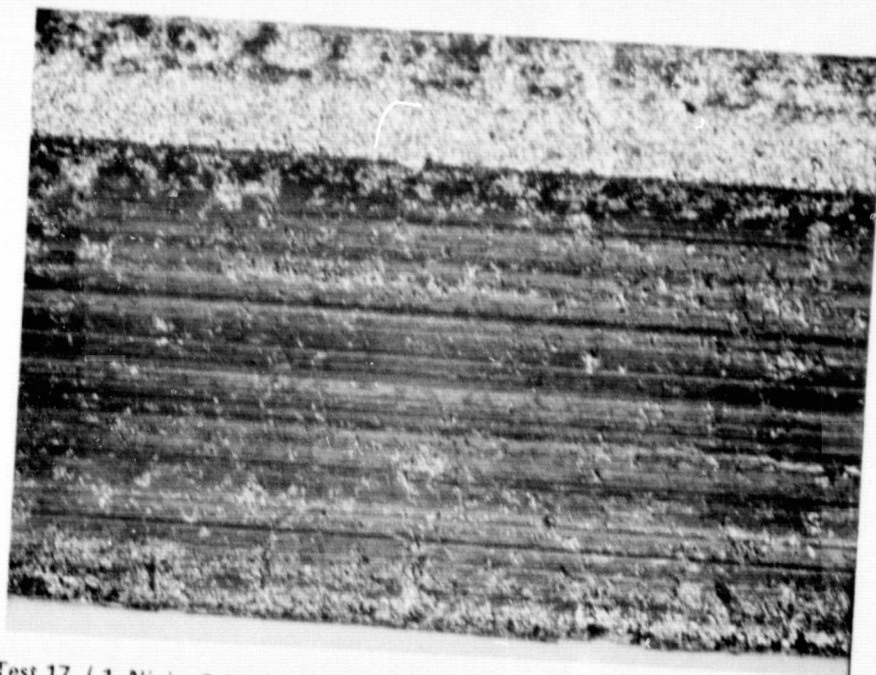
Figure 53. Seal Surface from Test 17 Showing Heavy Surface Glazing (Mag: 10x)
