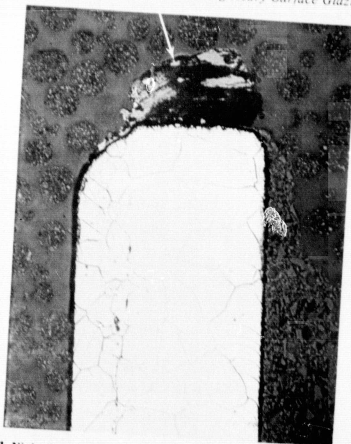
Test 13 ( 1, Ni, i = 0.25 mm/sec, v = 213 mps, b = .48 mm, \delta = 1.0 mm, \rho = 16\% )
