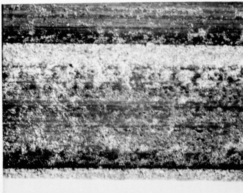
Test 14 ( 3, Ti, i = 0.25 mm/sec, v = 152 mps, b = 0.55 mm, \delta = 1.0 mm, \rho = 19\% )
