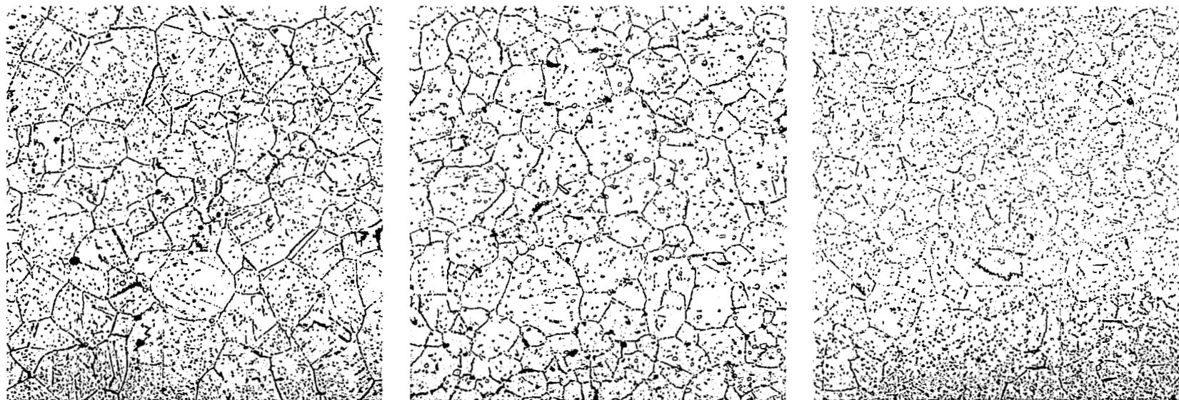
Figure 36: Optical Photomicrographs of Baseline Sheets after Creep Testing at 1200K/41.4 MPa (1700°F/6 ksi): (a) Heat 2-1604, (b) Heat 3-1622, (c) Heat 4-1671. Test specimens were oriented transverse to the rolling direction. X300.
