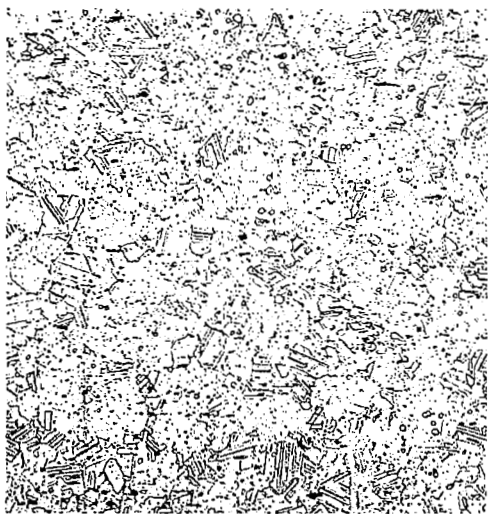
(a) 8A - 1394K (2050°F)/10 min. Grain Size ASTM 9-10 & Finer. X300.
