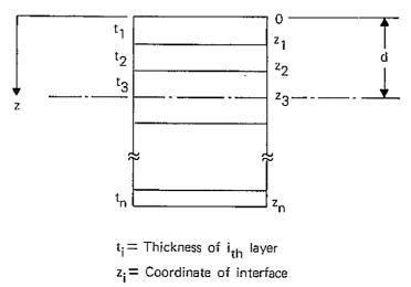
Fig. 1 - Cross Section of n layer Composite Beam
