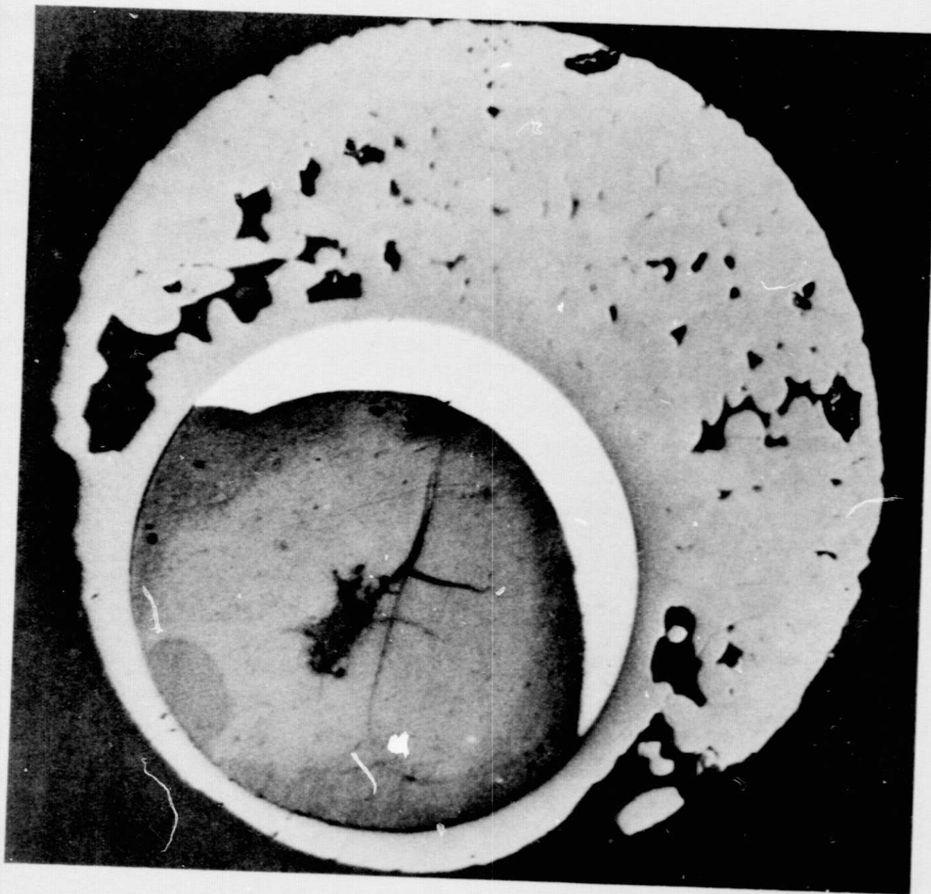
Fig. 6. An iron sphere with an eccentric Ni-rich core. The outer shell is magnetite. The bright rim of the core is Ni-Fe metal. The dark interior of the core is Si, Ni-rich trevorite. Scale = 25 \mu m.
