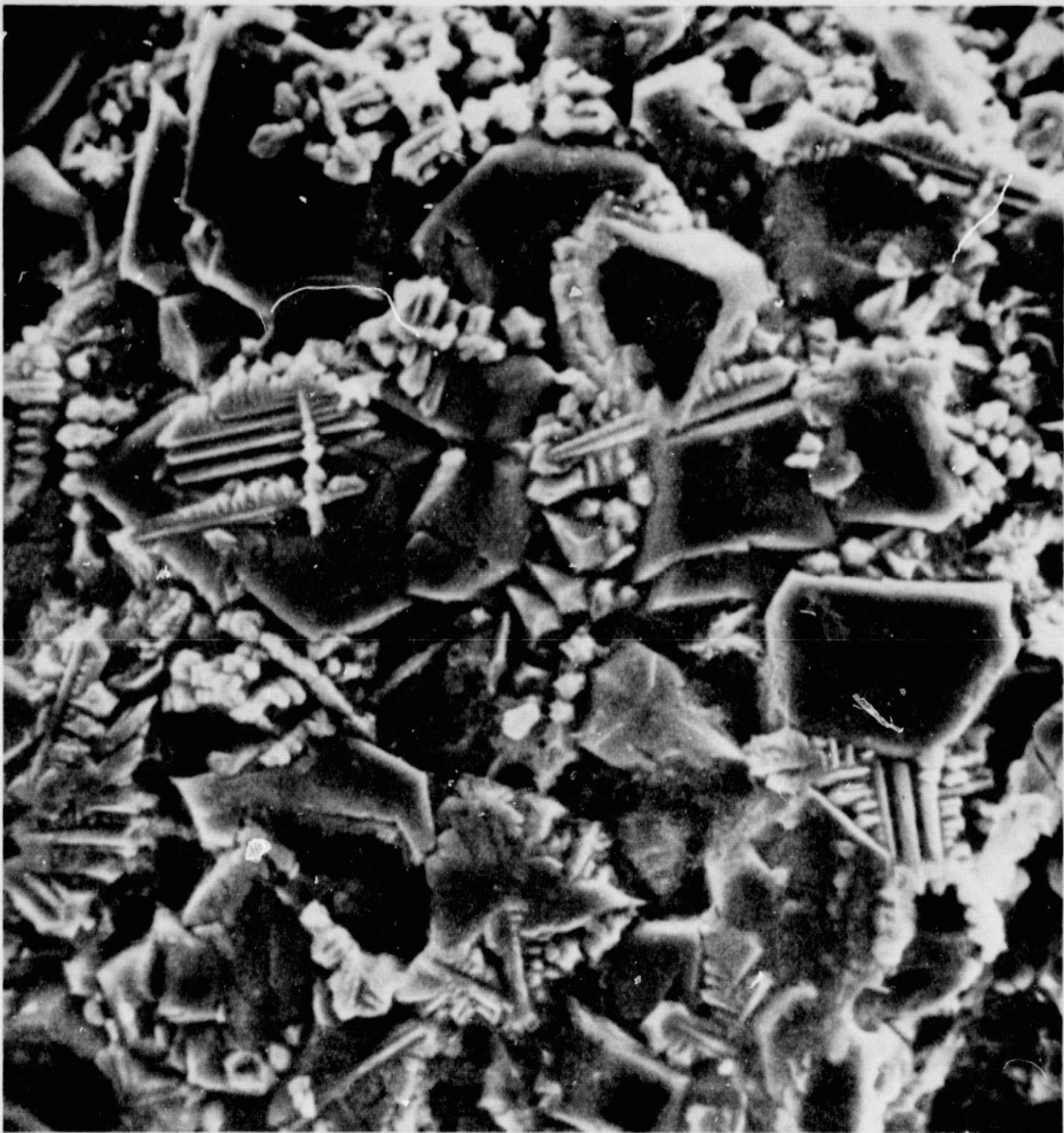
Fig. 8. Enlarged area of sphere shown in Fig. 1. Large crystals (gray) are olivine, small (bright) crystals often connected in chain-like fashion are magnetite, and groundmass areas are interstitial glass. Slightly above and to the right of the photo center is a hollow olivine crystal which has had its Mg-rich core dissolved away. Scale = 10 \mu m.
