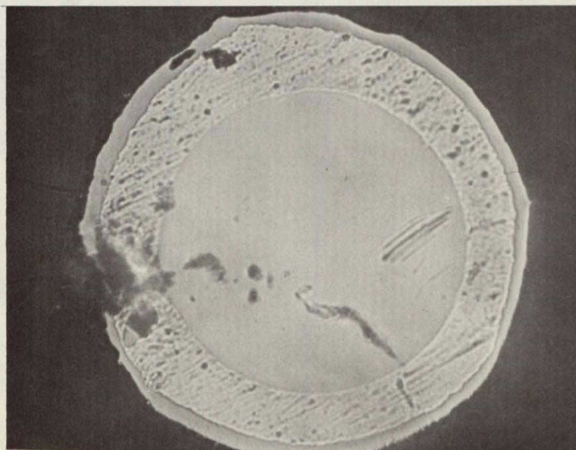
(c) Cross-section of wire electroless plated with 0.3 mil nickel 375°F heat treated used in runs 77-S through 79-S
