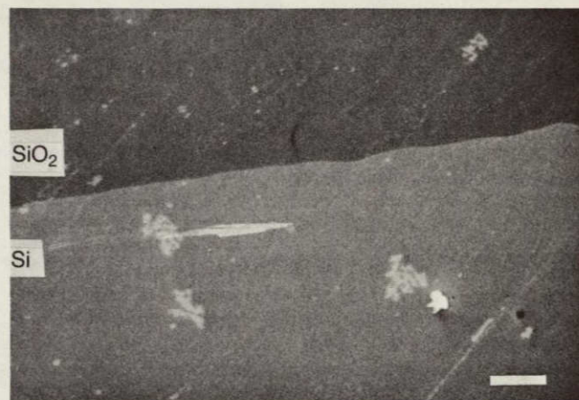
Fig. 2. Section of SiO 2 /Si interface showing strong bonding (10 kV, bar=10 \mu m).
