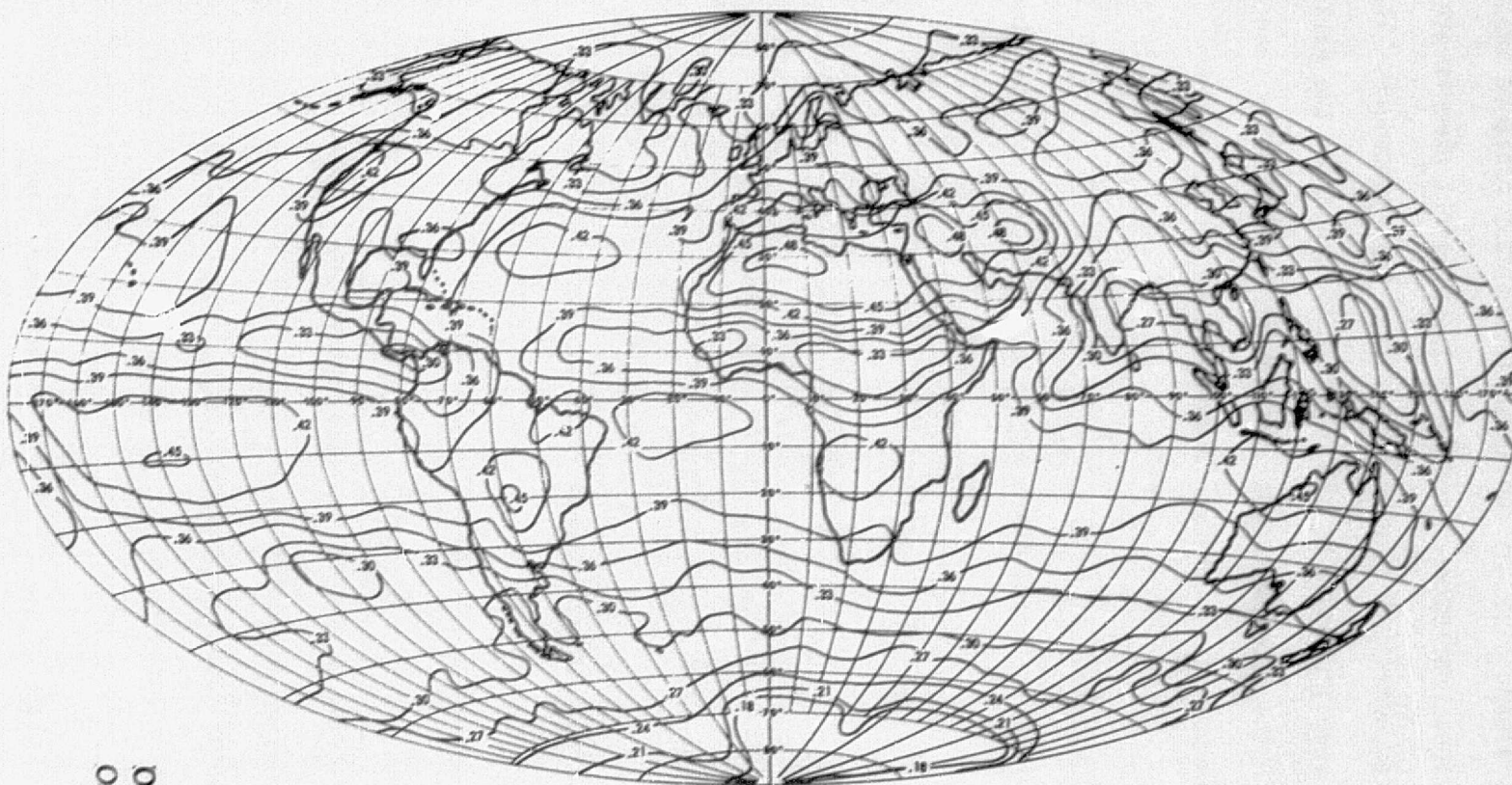
Figure 3. Emitted flux ( \text{cal/cm}^2 \text{ min} ) from the Earth-atmosphere system during the period July 16-21, 1969.
