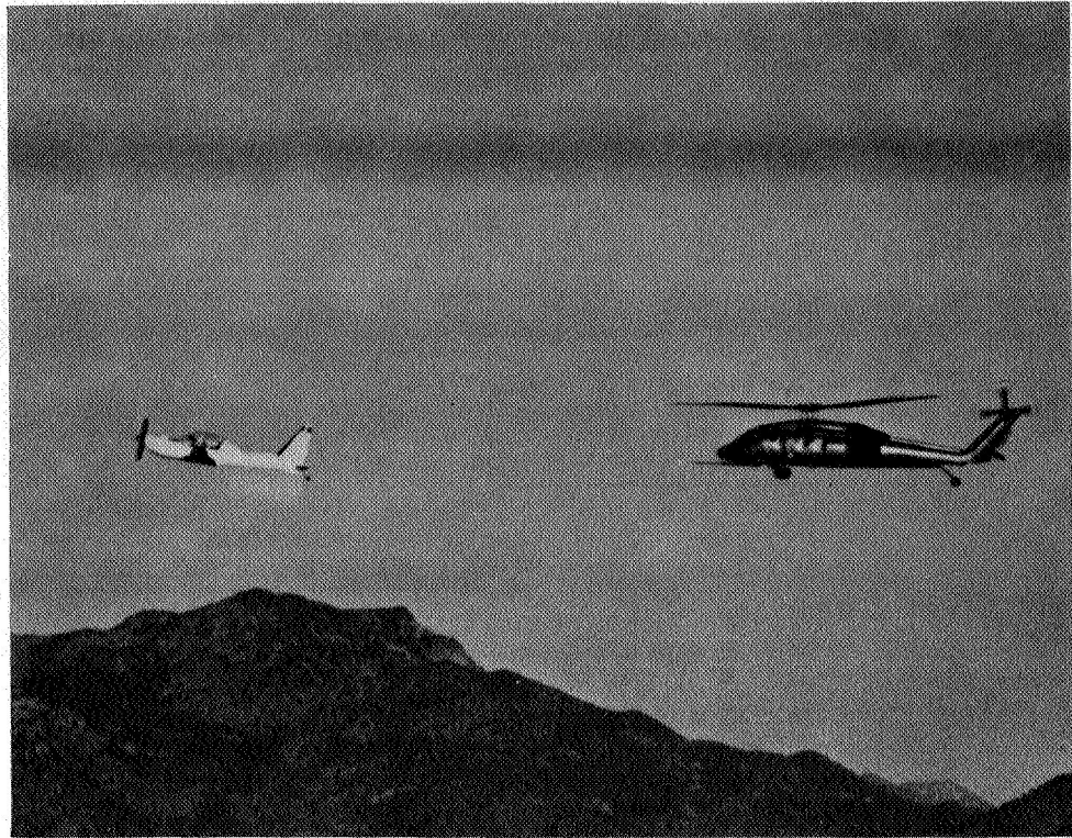
Figure 8.- YO-3A gathering acoustic data on Sikorsky UTTAS.
