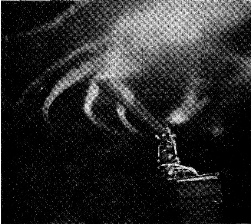
Figure 16.- Model UH-1H rotor interacting with previous tip vortices.
