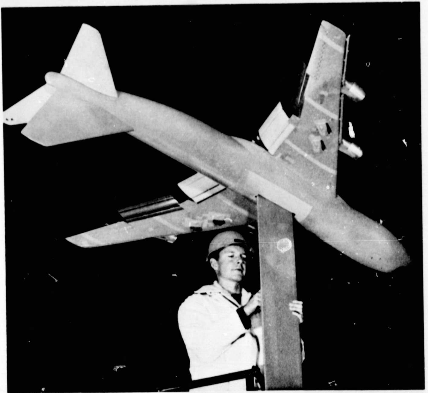
(c) Closeup view of B747 model tunnel with two circular arc fins mounted on each wing.
