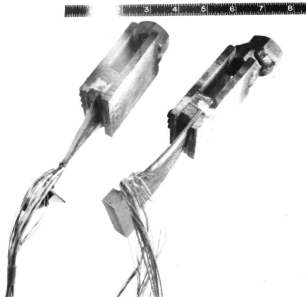
Figure 2-29 Titanium (L) and Steel (R) Test Specimens for Static Test With Transducer Mounting Configuration "E". Oblique view with tip fixtures installed. (77-441-9559-G)
