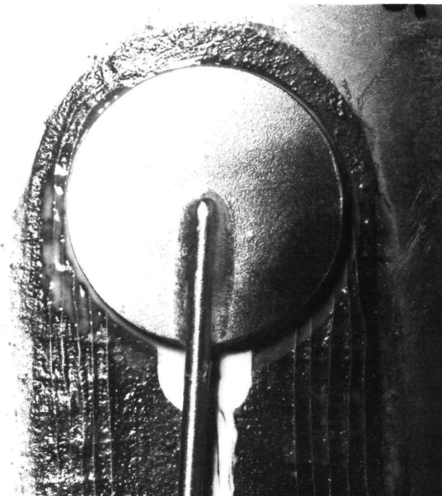
Figure 2-25 Titanium Test Specimen for Static Test With Transducer Mounting Configuration "C". View of transducer area on measured surface with pressure cap installed. Cap diameter is 19 mm and tube diameter is 1.57 mm (77-441-9321-A)
