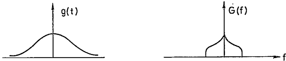
a. A time domain waveform g(t) and the corresponding frequency domain spectrum G(f)
