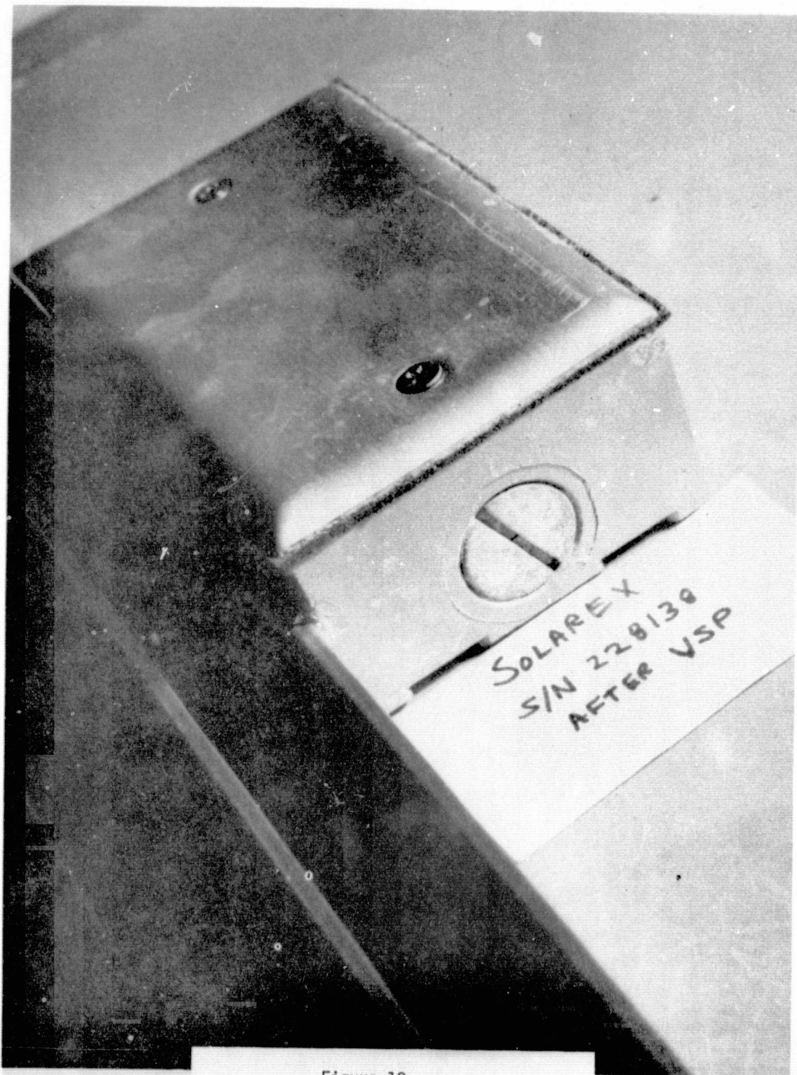
Figure 18 Corroded Plug in Terminal Box of Solarex Module Following Vacuum/Steam/Pressure
