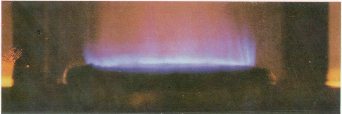
Working pressure, 20 atm; reactant velocity, 3 cm/sec
