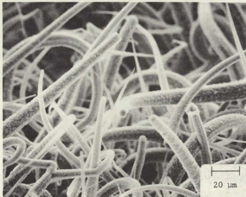
Figure 2-40. SEM Photograph of CVD Si Deposit on O-I Glass GS211 at \sim 850^{\circ}\text{C} in \text{H}_2 Atmosphere
