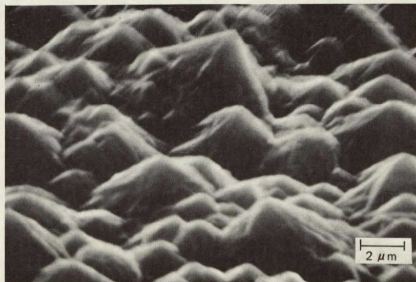
Figure 2-83. SEM Photographs of CVD Si Film Grown by \text{SiH}_4 Pyrolysis at \sim 840^\circ\text{C} in He on Substrate of Corning Code 9606 Glass-ceramic. a) and c) Viewed at 30 deg with Surface, b) Normal Incidence
