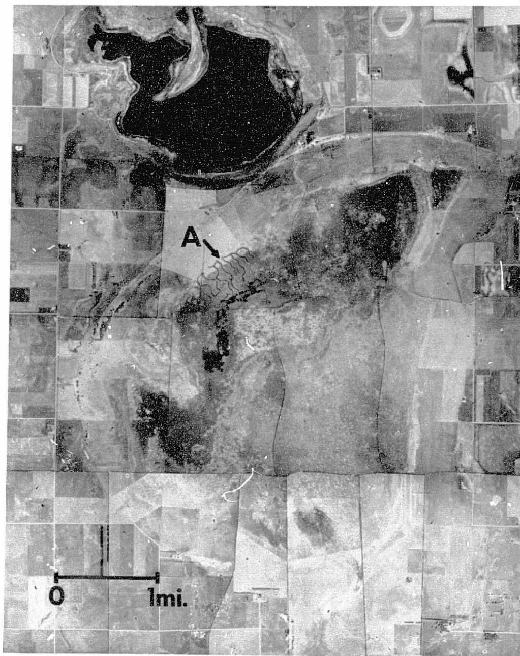
Figure 4. Photomosaics of Lake Thompson in Kingsbury County used for planning of level ditching project "B". Level ditching scheme at "A" was completed several years prior to data collection.
