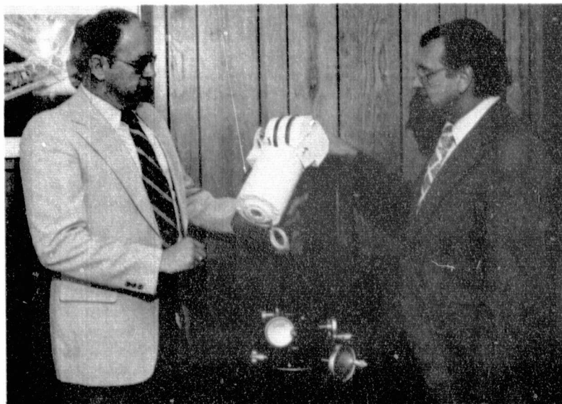
TRIPLE AXIS WRIST — Dwight Johnston (left), EEO1, examines a prototype TACPAW delivered to the Marshall Center on Aug. 1 by Dr. Leendert Kersten (right) of the University of Nebraska. The device is ready for integration with a seven-degree-of-freedom protoflight manipulator.
