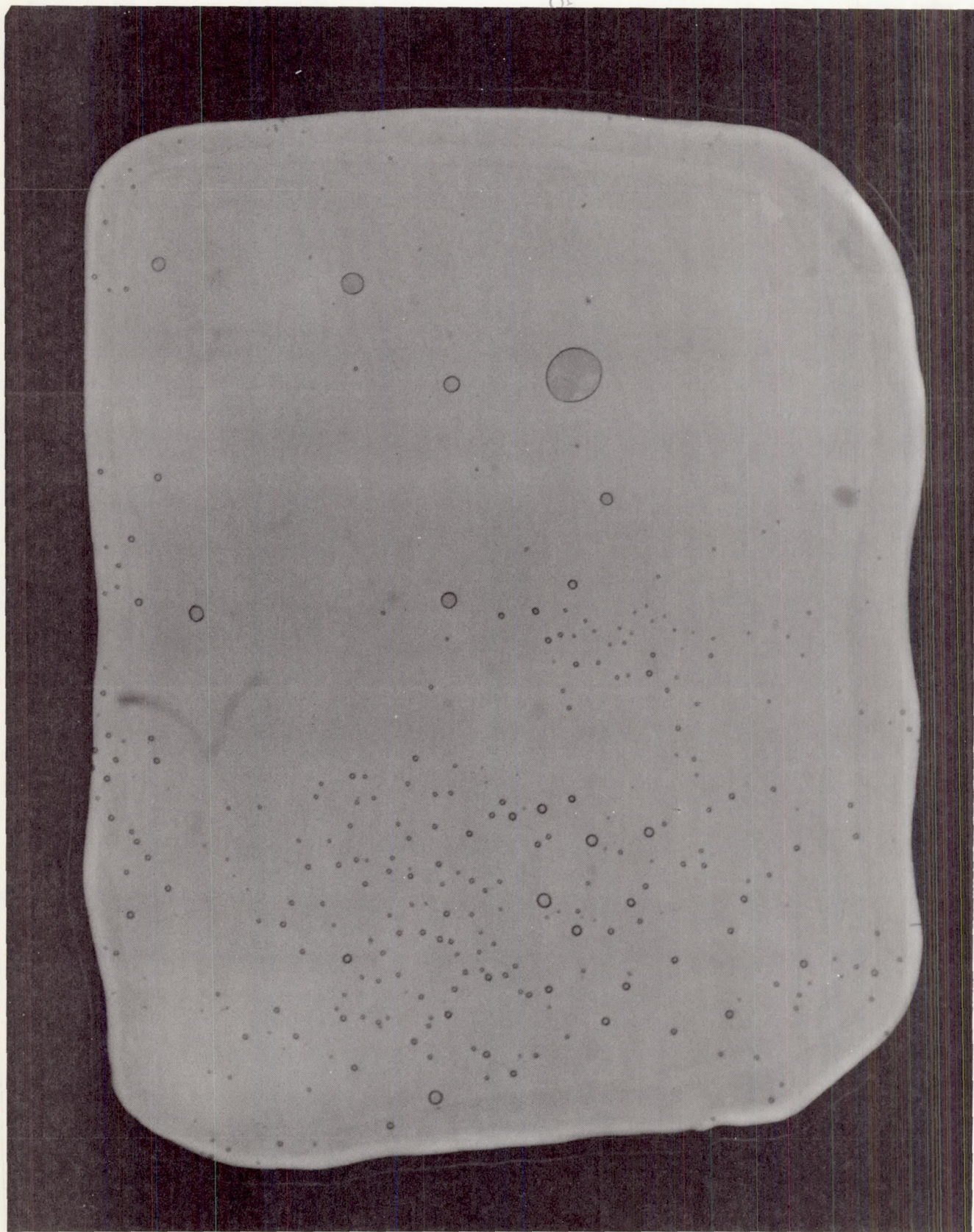
Figure 11 Uniformly Thinned 250 x 400 Membrane
