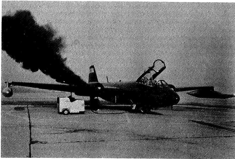
Fig. 22. B-57 airplane modified by the NACA Lewis laboratory to use liquid hydrogen in one engine. The wing-tip pod on the right (the airplane's left wing) is the hydrogen tank; the opposite pod contains helium for pressurization and purge. The dense smoke is normal in starting this engine on conventional fuel.
