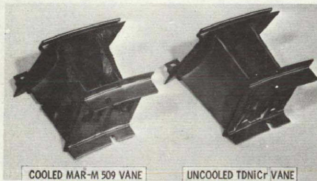
Figure 9. - Superiority of ODS vanes at overtemperature conditions.
