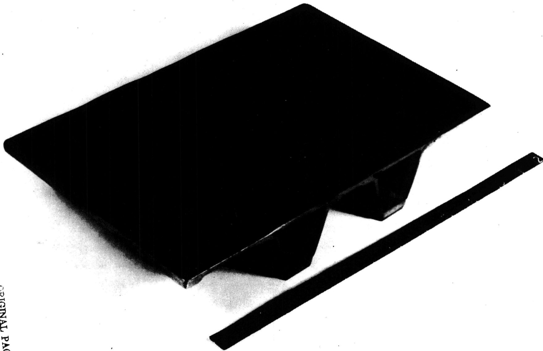
Figure 46 Final Demonstration Panel - Hat-Stiffened Semi-Sandwich
