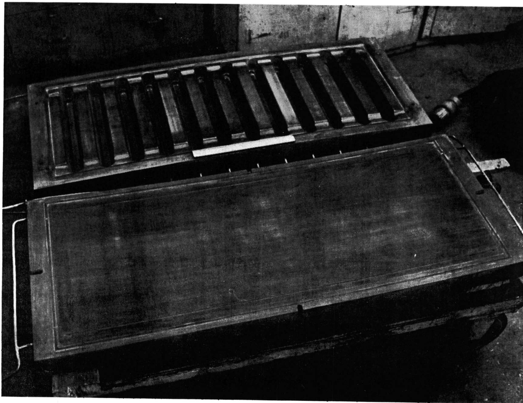
Figure 55 Feasibility Panel SPF/DB Tooling
