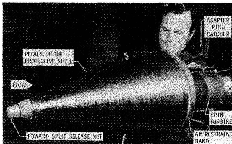
Figure 3.- Assembled model in test section of wind tunnel.
