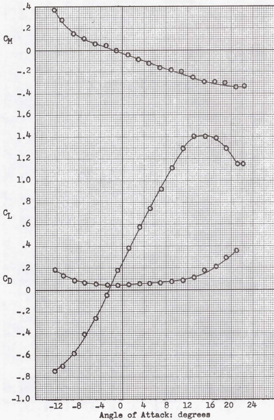
Figure 6.- Aerodynamic characteristics of the semi-sailwing model 2.
