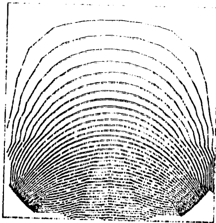
Figure 7. - Equipotential lines for boundary value problem.
