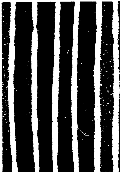
Figure 1. Layered composite material niobium- \text{Al}_2\text{O}_3 (cross section: 50 x magnification)
