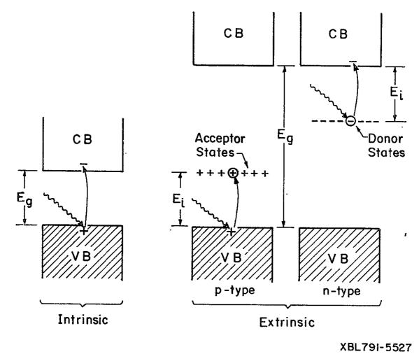
semiconductor and of the particular dopant. Of special interest are extrinsic detectors in silicon and germanium denoted generically Si:XX and Ge:XX (where XX represents any of a number of dopants). These are clearly the best available photon detectors for  $15~\mu m < \lambda < 210~\mu m$ .
