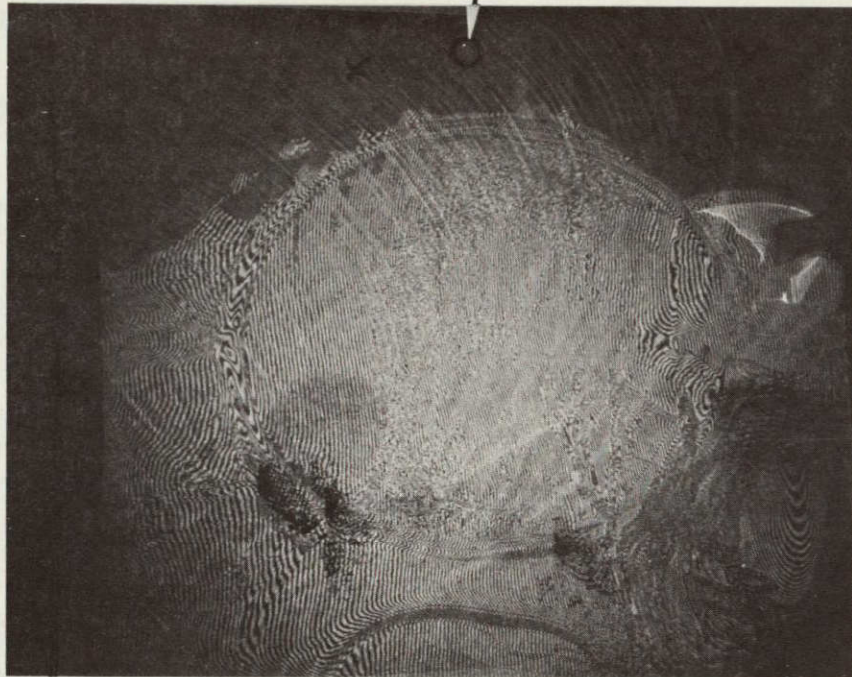
FIGURE 1. COHERENT-LIGHT IMAGE OF SEVERELY DELAMINATED ACRYLITE-SCOTCHWELD ENCAPSULATED CELL
