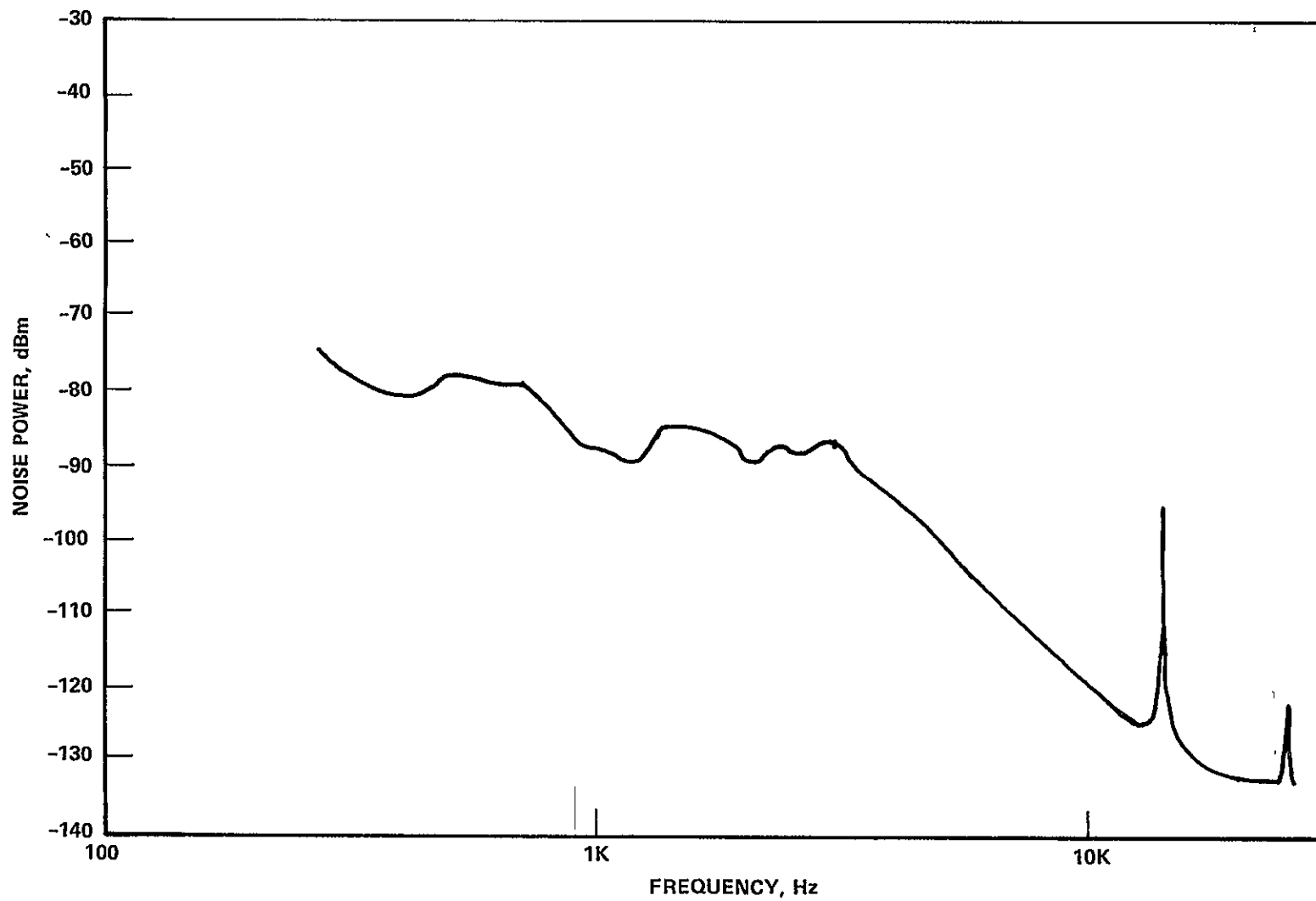
FIGURE 29. NOISE CHARACTERISTIC OF CELL #411 OVER THE RANGE 200 Hz – 25 kHz; BANDWIDTH 100 Hz
