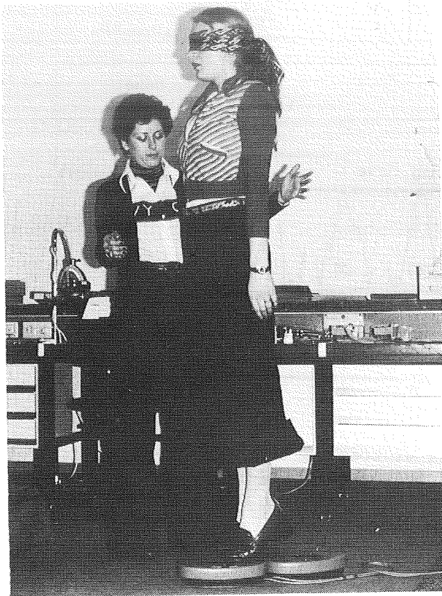
Figure 5.- Test person on the scales. She is balancing on toes or heels with covered eyes and ears.
