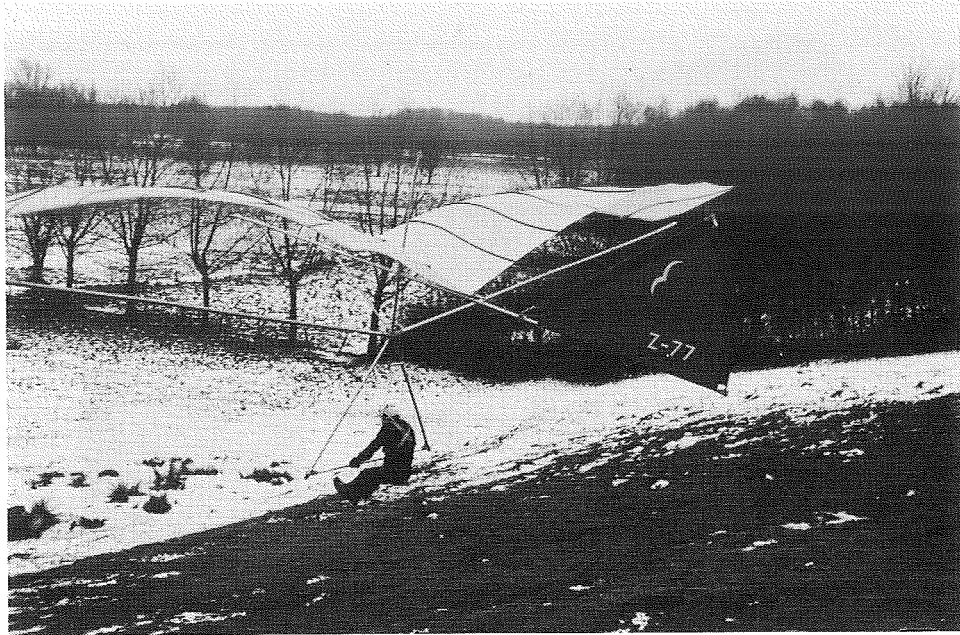
Figure 5.- Experimental hang glider Z-77 (first variant) with cable leading edge elastic wing.
