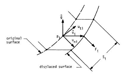
According to the Lagrangian formulation which is used in structural mechanics, the force on the structural interface is equal to the integral of the pressure over the <u>displaced</u> surface, which, to first order in small quantities, equals the pressure on the original surface plus a term due to the gravitational force on the fluid between the two boundaries. Thus the force on the boundary structural grid point in the direction of the normal is, assuming small motions,
