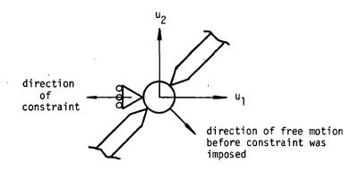
The direction of constraint allows the point to move only vertically, but, since the rods are collinear, the force of constraint is zero and the forces in the elements are still valid. The NASTRAN system detects singularities of individual grid or scalar points during problem formulation, see Section 3.4. As in the above example, more than one valid way exists for constraining a geometric grid point. The possible constraints are listed in a warning message in their order of preference.
