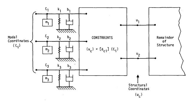
Figure 1. Representation of part of a structure by its vibration modes when all connection points are free while the modes are calculated.
