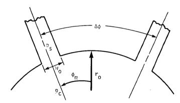
We might, for example, assume that the pressure in the mouth of the  $m^{th}$  slot,  $p_{s,m}$ , is equal to the pressure in the cylindrical region evaluated at  $\phi = \phi_m$ , the midpoint of the slot. A better assumption, particularly for wide slots, is that  $p_{s,m}$  is equal to the <u>average</u> pressure in the cylindrical region, averaged over the slot width. Thus, using Equation 1, the pressure in the width of the  $m^{th}$  slot is
