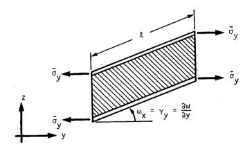
Figure 2. Shear deformation of a sandwich plate.
