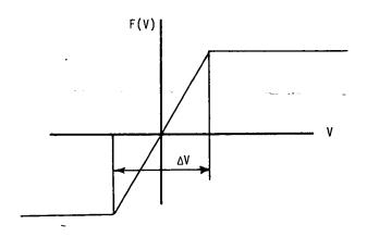
Figure 2. Recommended force-velocity curve for coulomb damper.
