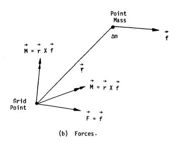
Figure 1. Accelerations and forces on a rigidly connected point mass.
