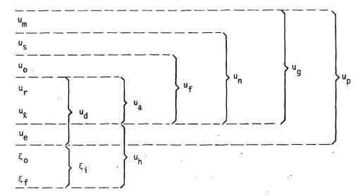
In static analysis we are concerned only with the grid point set,  $\{u_g\}$ , and its subsets. The application of constraints and partitioning to the stiffness matrix involves, essentially, the elimination of  $\{u_m\}$ ,  $\{u_s\}$ ,  $\{u_o\}$  and  $\{u_r\}$  from  $\{u_g\}$  to form a stiffness matrix referred to  $\{u_g\}$ .
