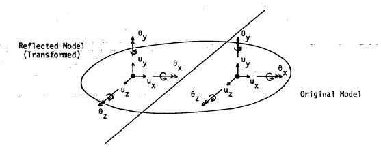
All subsequent combinations using this new substructure would proceed as for any other substructure. On data recovery, however, the user must be careful. The detailed results obtained for the basic reflected model (Phase 3) will be output in the <u>reflected</u> coordinate system and, therefore, must be interpreted with the <u>left-hand</u> rule. These results, of course, include not only displacements and rotations at grid points, but they also include stresses and element forces and moments.
