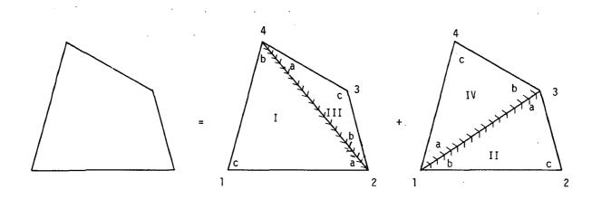
For each triangle the x-axis lies along a diagonal so that internal consistency of displacements and rotations of adjacent triangles is assured. Each triangle has one-half of the bending stiffness assigned to the quadrilateral.
