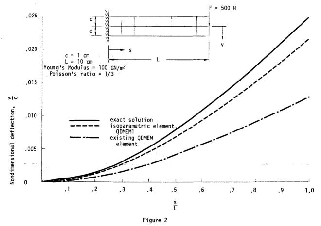
Deflection of cantilever beam idealized by quadrilateral membrane elements
