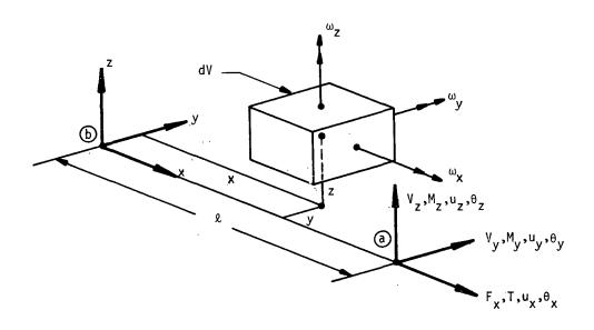
All forces, moments, displacements and rotations follow right-hand rules. The rotations of an infinitesimal element located within the beam are also indicated in the figure.
