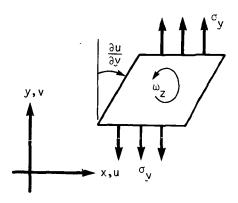
Figure 3. Shear deformation of a unit cube.
