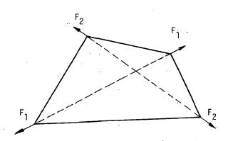
Forces  $F_1$  and  $F_2$  are evaluated from corner displacements during stress data recovery (see Section 5.3). The diagonals are treated as independent extensional rods, for the purpose of calculating differential stiffness. The resulting matrices are then transformed from element coordinates, which are oriented parallel and perpendicular to the diagonals, to grid point coordinates. Details of the procedure are described in Section 8 of the Programmer's Manual.
