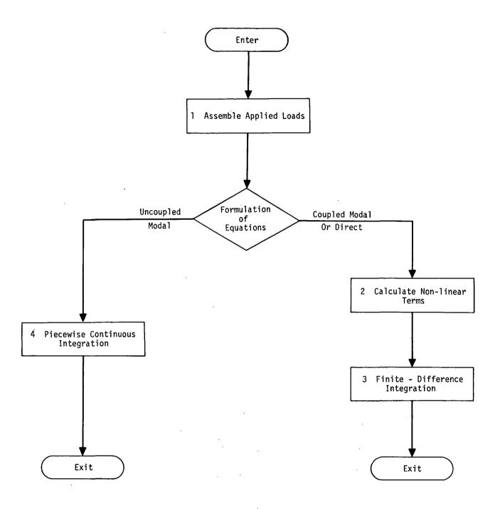
Figure 1. Simplified flow diagram for transient analysis module, TRD.
