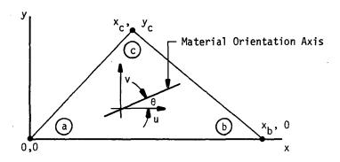
Figure 1. Triangular Membrane Element
