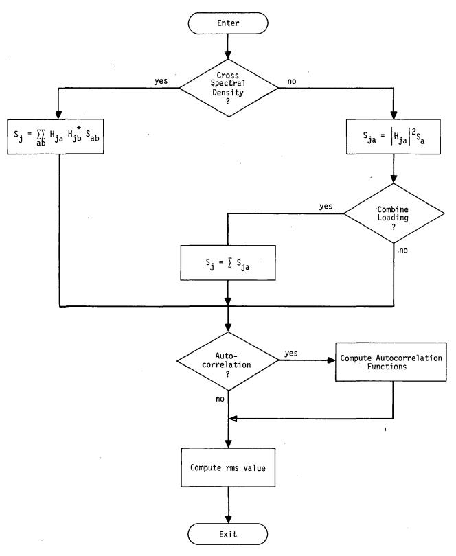
Figure 1. Flow diagram for random analysis module.
