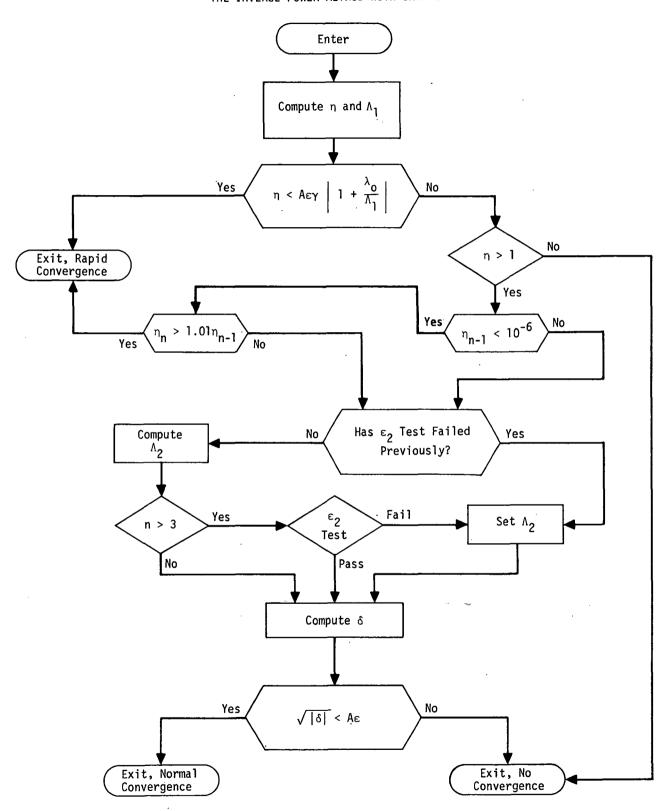
Figure 3. Flow diagram for block 4.3, convergence tests.
