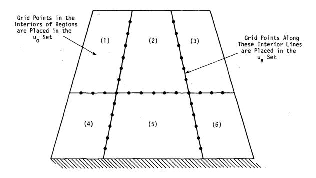
Figure 1. Use of partitioning to decouple regions of the structure.
