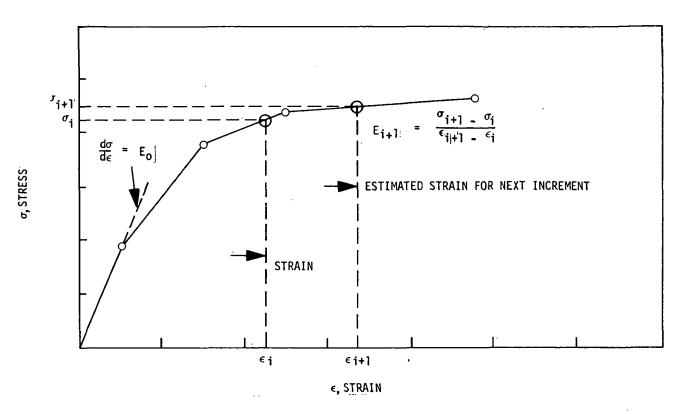
Figure 2. Determination of elastic modulus from tabular stress-strain curve defined by user.
