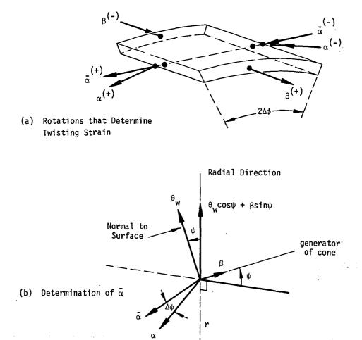
Figure 2. Geometrical relationships used in calculation of twisting strain.
