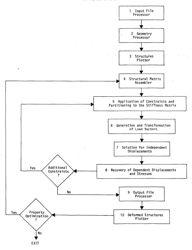
Figure 1. Simplified flow diagram for Basic Static Analysis.
