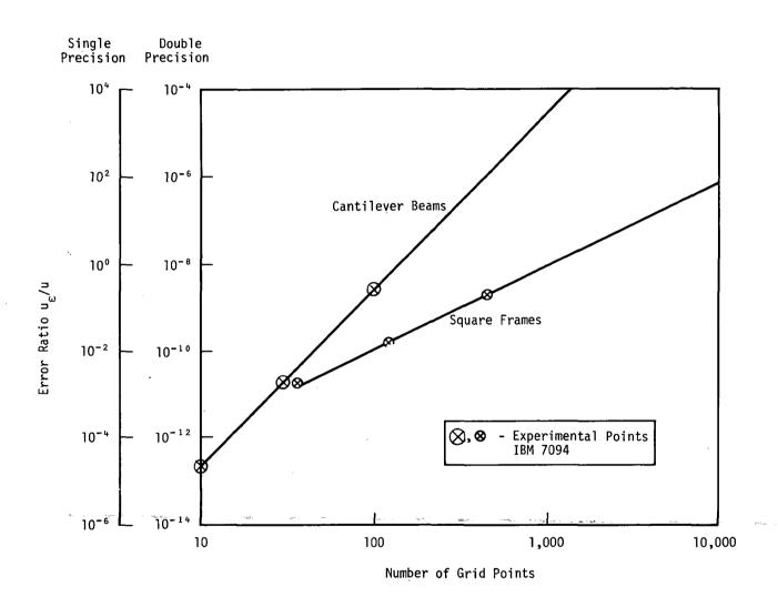
Figure 2. Effect of roundoff error in static solutions.
