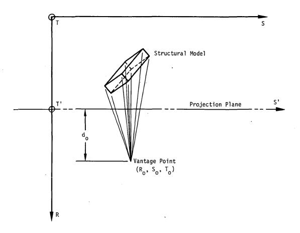
Figure 3. Perspective projection geometry.
