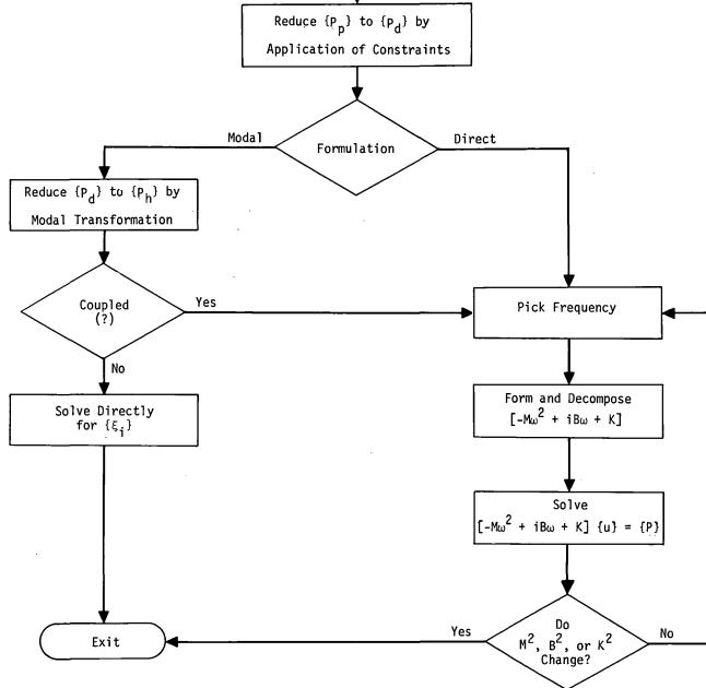
Figure 1. Flow diagram for frequency response module, (FRD).
