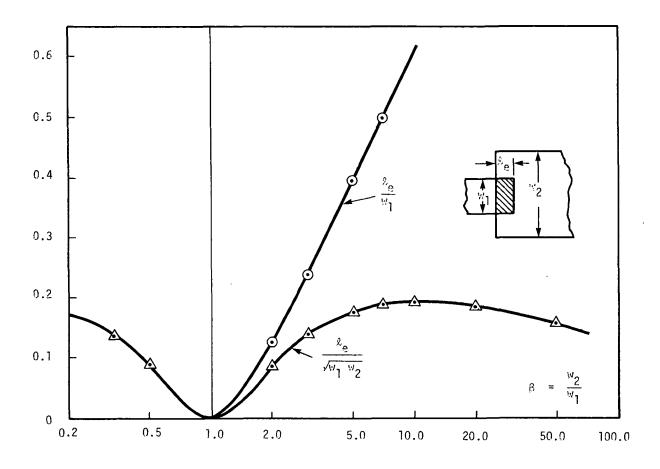
Figure 5. Effective length of an abrupt change in the width of a strip.
