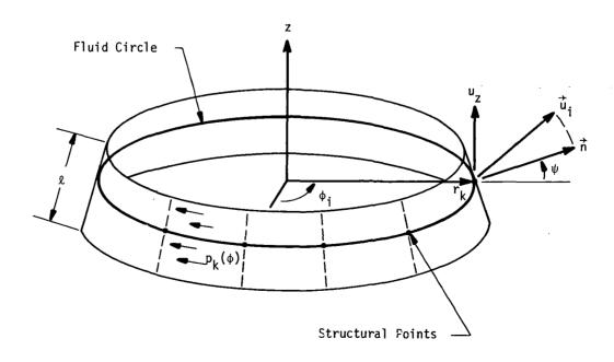
$\ell$  is the slant length of an equivalent conical surface associated with the circle
