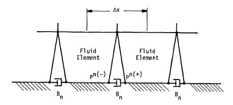
Each fluid grid point on the boundary is replaced by a pair of closely spaced grid points, between which a viscous damper,  $B_n$ , is connected for each harmonic order. One, but not both, of each pair of fluid grid points is identified as lying on the structural interface.
