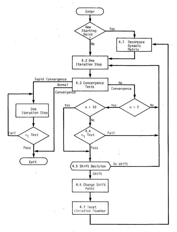
Figure 2. Flow diagram for block 4, compute one eigenvalue and one eigenvector.
