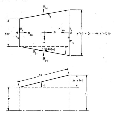
The positive direction of moments shown above is consistent with the positive convention for curvatures.
