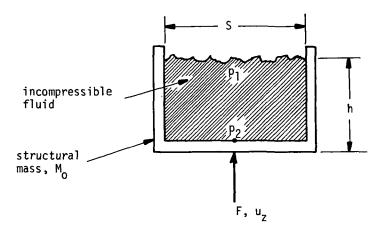
Compute the vertical motion  $\boldsymbol{u}_{\boldsymbol{z}}$ , in response to an oscillating vertical applied force, F.
