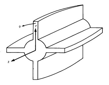
Figure 1. Symmetrical acoustic cavity with slots.
