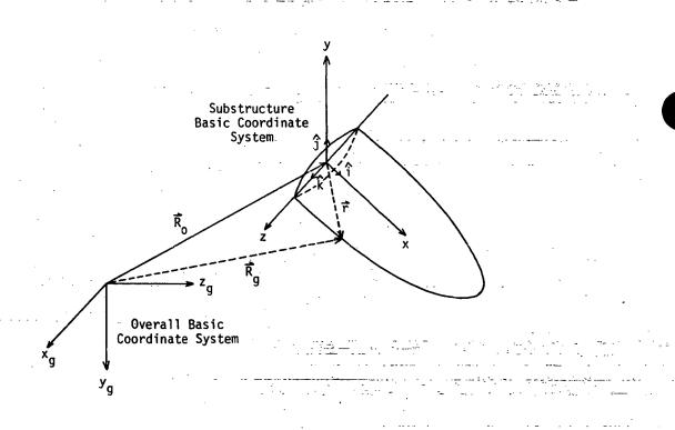
The locations of the substructure points in the overall basic coordinate system are described by the equation:
