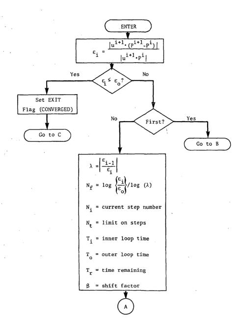
Figure 2a. Flow diagram for module DSCHK (first part).
