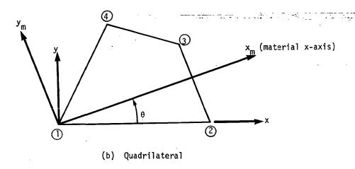
Figure 1. Material axes for surface elements.
