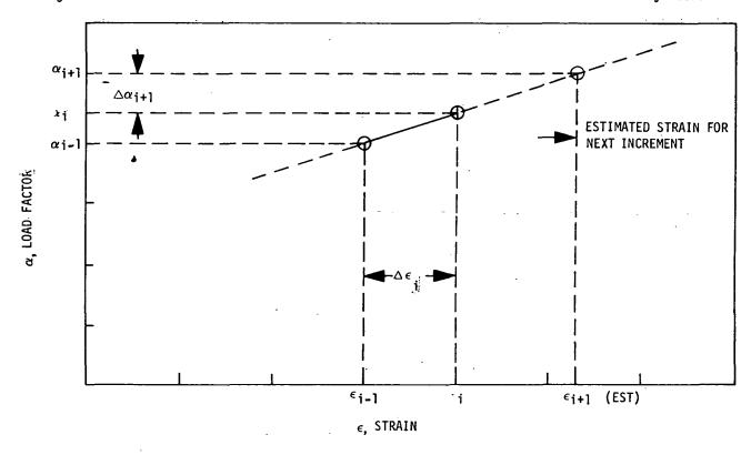
Figure 3. Method of extrapolating previous strains to produce estimate of next strain.
