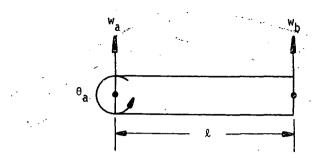
A multipoint constraint also applies forces,  $q_{cg}$ , to each of the degrees of freedom included in the equation of constraint, Equation 1. A double subscript is used to indicate the force on the gth degree of freedom due to the cth constraint. The forces are proportional to the coefficients,  $R_{cg}$ , in Equation 1, as will be shown. Thus
