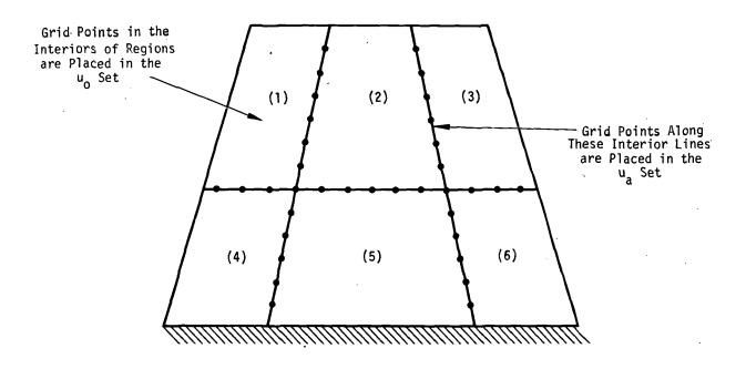
Figure 1. Use of partitioning to decouple regions of the structure.
