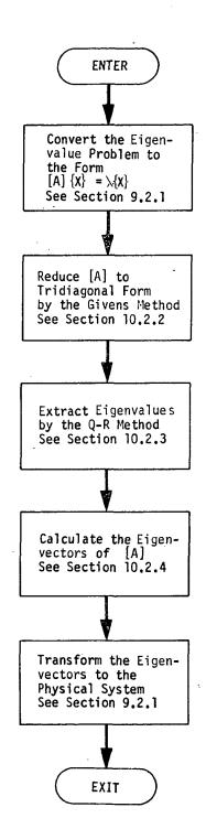
Figure 1. Simplified flow diagram for the tridiagonal method.
