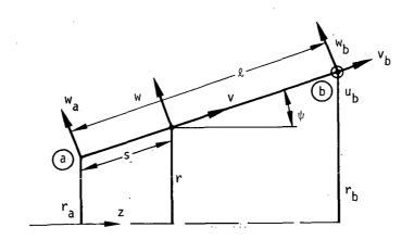
Figure 1. Coordinate geometry for conical shell element.
