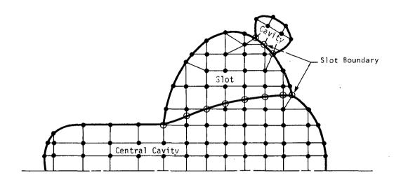
Figure 4. Finite element model of acoustic cavity.
