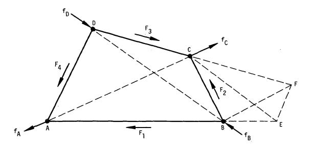
Figure 1. Shear panel and its force polygon.
