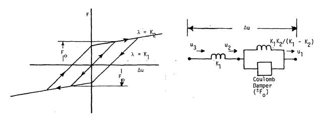
Figure 3. Plastic deformation element.
