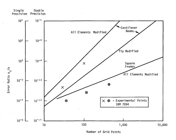
Figure 1. Effect of stiffness matrix error in static solutions.
