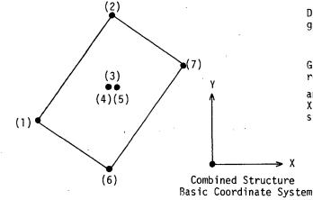
Displacement component in Y direction at grids 2 and 6 are  $\underline{\text{not}}$  to be connected.
