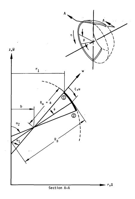
Figure 1. Toroidal thin shell ring representation.
