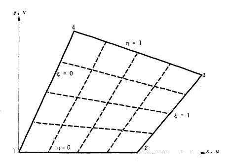
Figure 1. Coordinate systems for quadrilateral membrane element.
