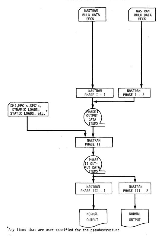
Figure 2. Flow diagram for NASTRAN substructuring.
