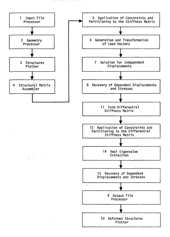
Figure 3. Simplified flow diagram for buckling.
