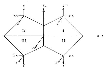
where the original basic substructure (I) was reflected in the x-z plane to create substructure (II). Substructures (I) and (II) were combined and subsequently reflected in the y-z plane to create substructures (III) and (IV) to complete the four part model. The final model would comprise four basic substructures, of which substructures II and IV would produce Phase 3 results in the left-handed coordinate systems as shown.
