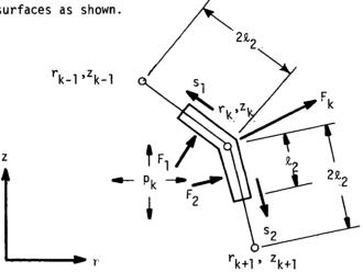
The forces on each of the two sections, for a unit increment of azimuth angle, are
