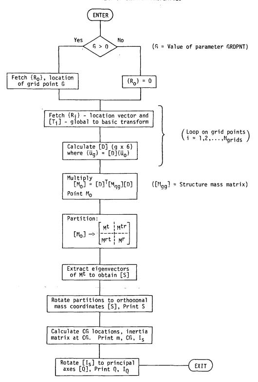
Figure 3. Flowchart of grid point weight calculations.
