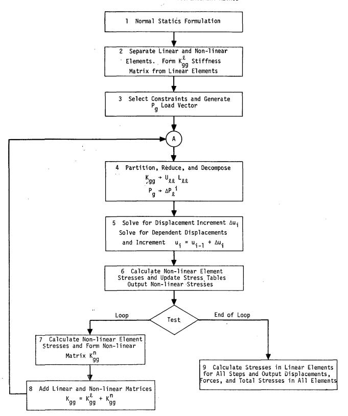
Figure 1. Piecewise linear flow diagram.
