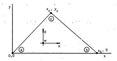
Figure 2. Coordinate Geometry for the Basic Bending Triangle
