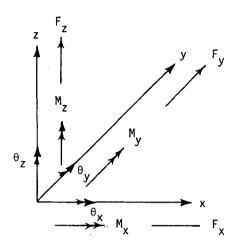
The mass associated with a grid point is assumed to be rigidly attached to, and in the vicinity of, the grid point, regardless of the elastic deformation. In effect then, the mass associated with grid point behaves as a local rigid body with the properties computed with respect to that grid point.
