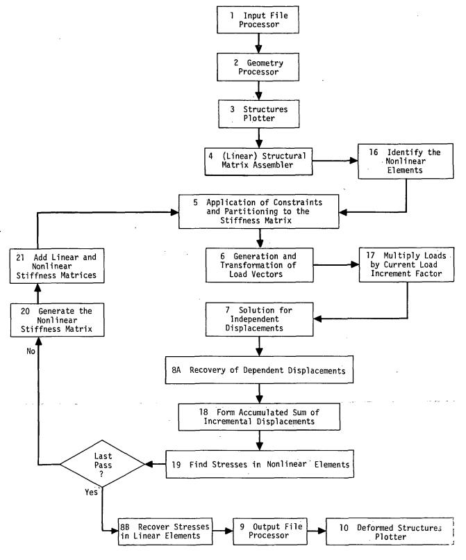
Figure 4. Simplified flow diagram for piecewise linear analysis.
