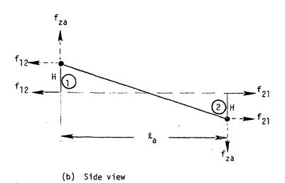
Figure 3. Method of transferring forces from a plane quadrilateral element to adjacent nonplanar grid points.
