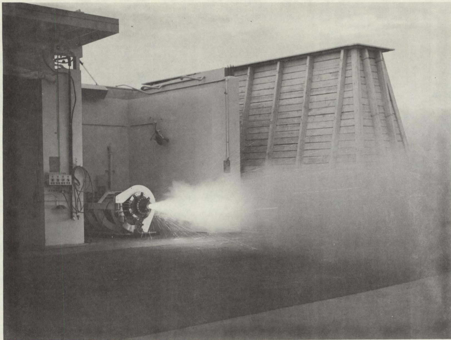
Figure 3-1. BATES Motor Firing of 0% AP in AN/AP/Al/HTPB
