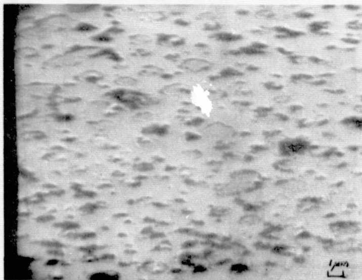
Figure 28. S009 (5 wt% AgF) on polished silicon fired at 750 C° in air, removed with \text{HNO}_3 . Tilt angle 15° at 4150X.
