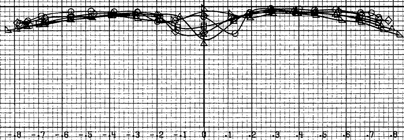
Figure A60. Effect of rotation rate and angle of attack on axial-force coefficient for T-tail configuration. \delta_a = 0^\circ , \delta_s = 0^\circ , \delta_c = -25^\circ , \beta = 0^\circ .
