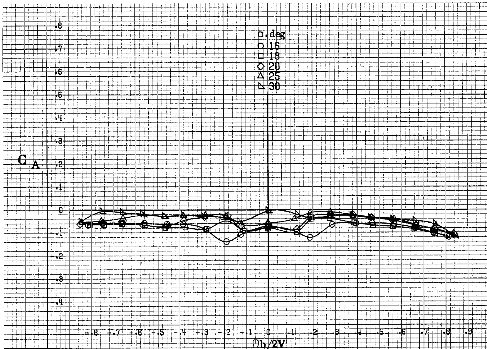
Figure A126.-Effect of rotation rate and angle of attack on axial force coefficient for configuration having outboard LE wing droop extended inboard 45.2cm(17.8in). \delta_s=0^\circ , \delta_a=0^\circ , \delta_r=0^\circ , \beta=0^\circ .
