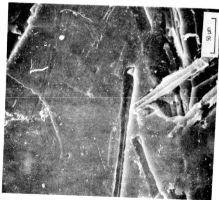
Figure 19. - Argon-ion textured high-molecular weight polyethylene with 10% carbon fibers, 300X.
