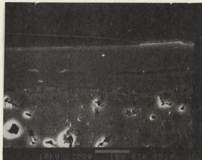
Fig. 12 Vitre-Graf coating on fine-grained graphite substrates: (a) six layers of light solution, and (b) four layers of heavy solution.
