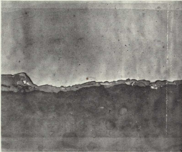
Fig. 1 Interface between mullite (lower) and silicon (upper) shows the Vitre-Graf coating intact and partially reacted with silicon to form a silicon carbide layer. (450x)
