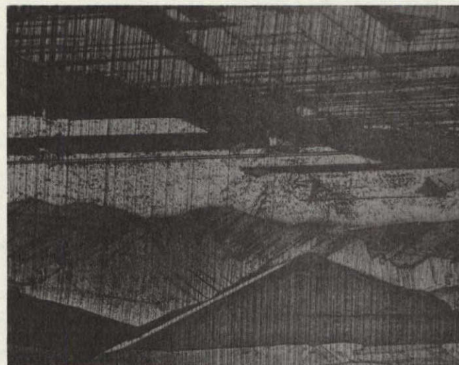
Fig. 16 Silicon dip evaluation: (a) silica substrate partially wetted with silica film; (b) grain structure of silicon film on mullite substrate coated with Vitre-Graf and cured at 1050°C; (c) fine-grained graphite substrate cured at 1150°C with heavy silicon film; (d) grain structure of silicon film on molded graphite substrate coated with Vitre-Graf and cured at 1150°C (a&c: 4x; b & d: 40x)
