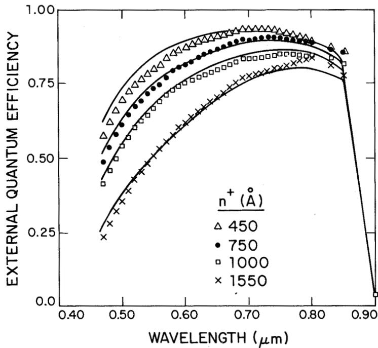
Fig. 4 External quantum efficiency as a function of wavelength for GaAs shallow-homojunction solar cells with n<sup>+</sup> layer thickness of 450, 750, 1000, and 1500 Å.
