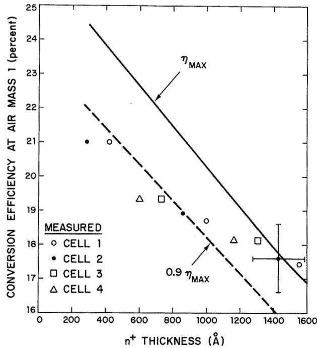
Fig. 5 Efficiency at AM1 as a function of  $n^+$  layer thickness. Measured values are represented by points, calculated values of maximum conversion efficiency  $\eta_{\text{MAX}}$  and of  $0.9 \eta_{\text{MAX}}$  by solid and dashed lines, respectively.
