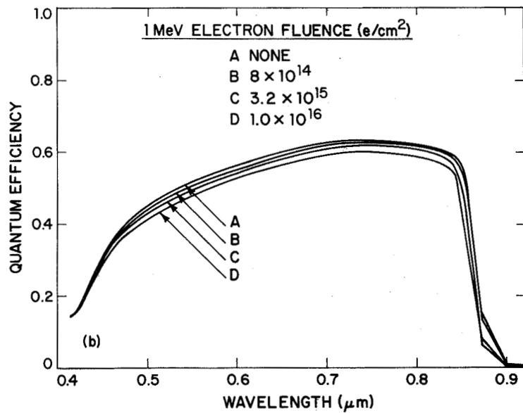
Fig. 7 a) The characteristics of Cell 2 as a function of cumulative electron fluence.
