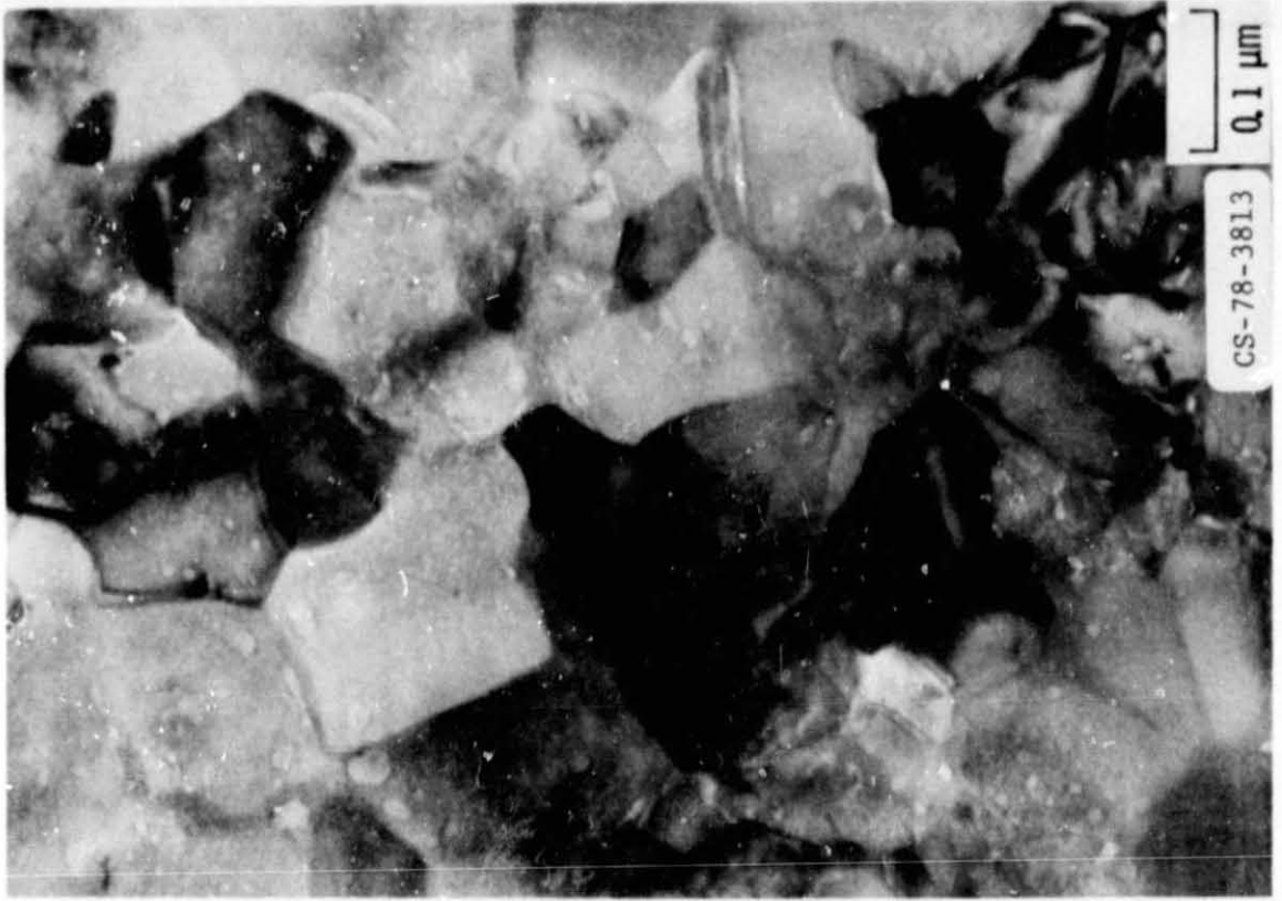
Figure 1. - Fine voids and grains in \alpha - \text{Al}_2\text{O}_3 scale formed on pure NiCrAl, 0.1 hr at 1100° C.
