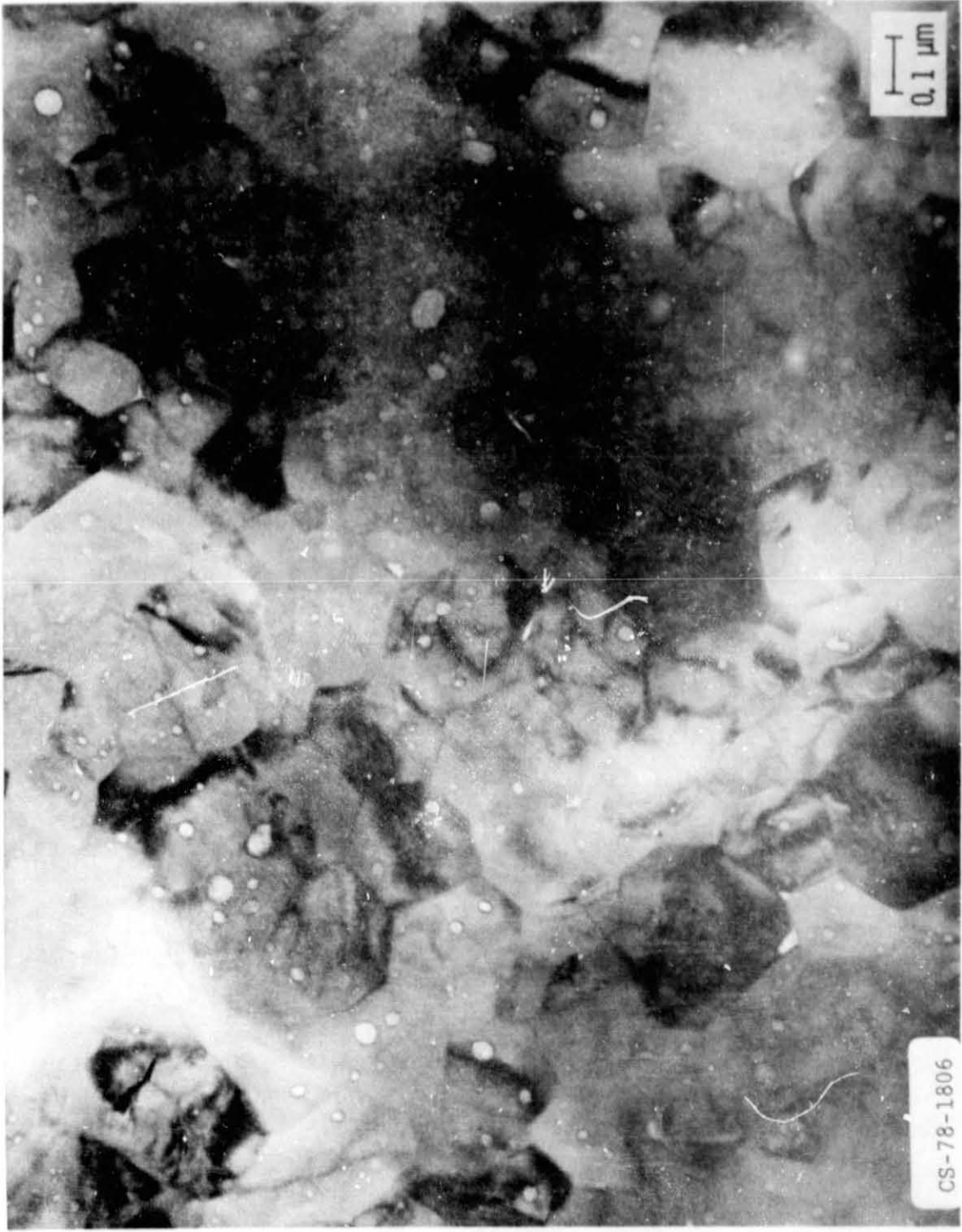
Figure 2. - Growth of voids and grains in \alpha - \text{Al}_2\text{O}_3 scale after 1 hr of oxidation.
