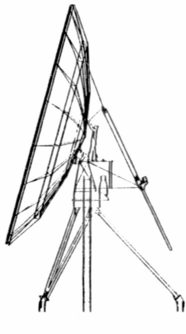
FIGURE 3-93. TYPICAL CONCENTRATOR INSTALLATION SEQUENCE (SHEET 2 of 2)
