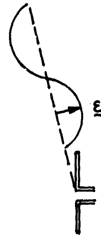
Figure 9b. Incident Electric Field on the Dipole
