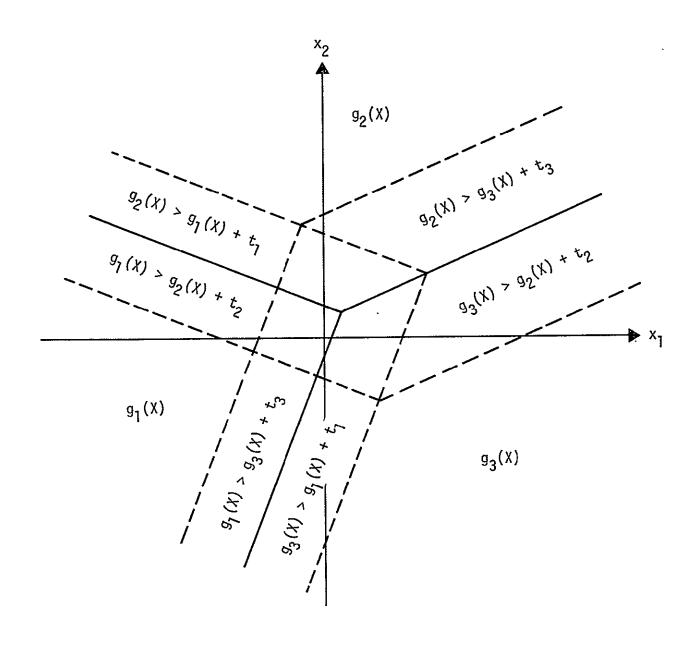
Figure 4-5.— Illustration of decision surfaces and thresholds.
