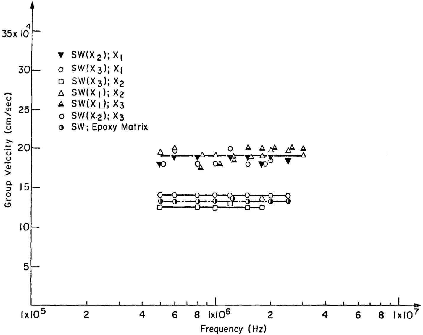
Fig. 11 Shear wave group velocities versus frequency for the indicated specimens and directions. (Specimens had 1.270 cm x 1.270 cm Cross Section.)
