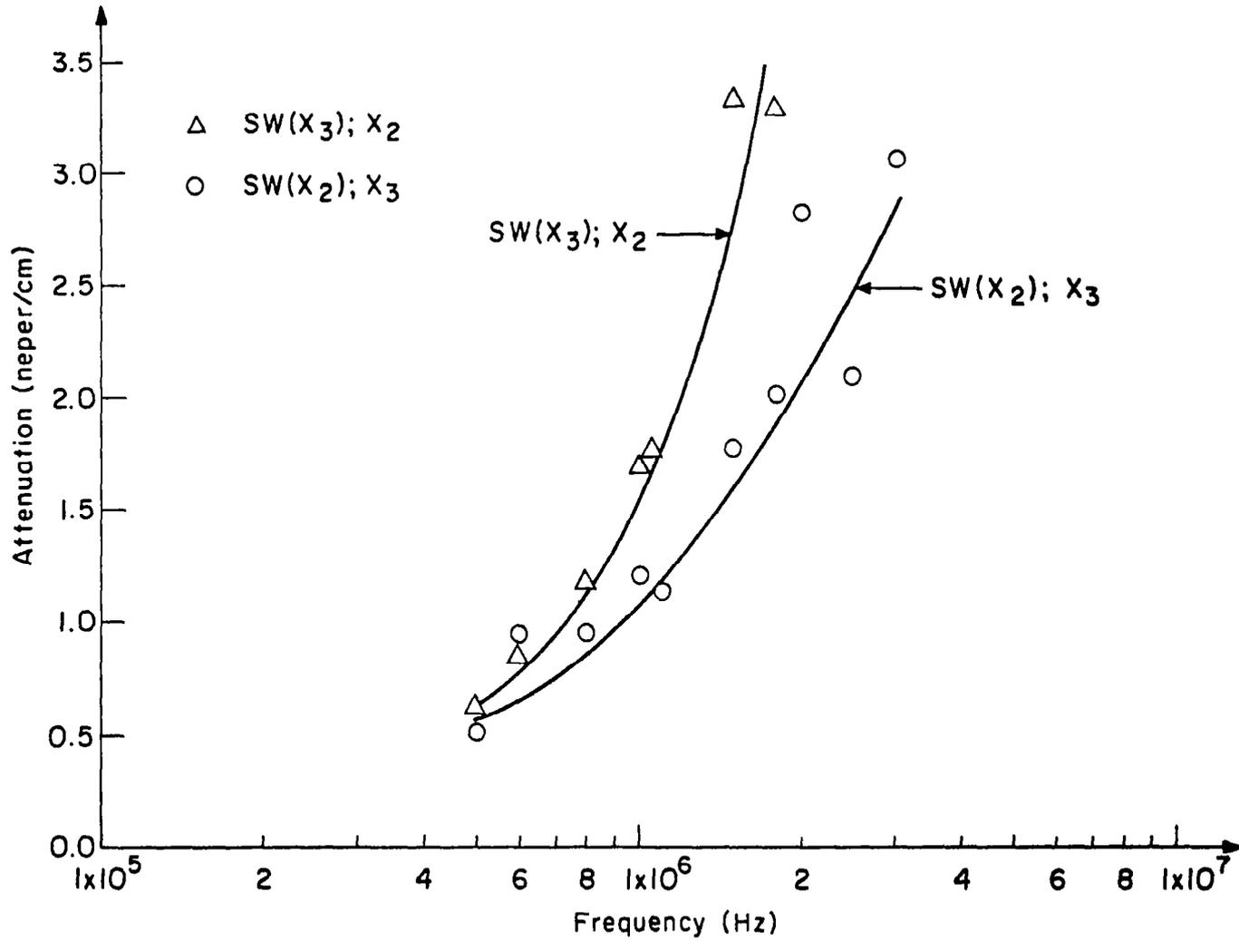
Fig. 13 Attenuation of shear wave in the indicated directions and specimens. (Specimens had 1.270 cm x 1.270 cm Cross Section.)
