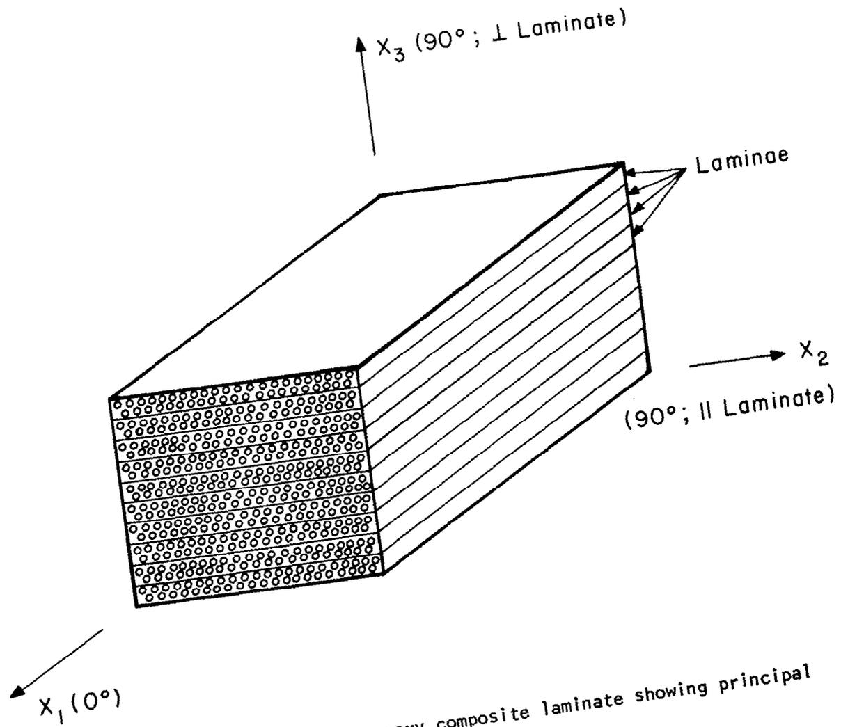
Fig. 1 Schematic of graphite epoxy composite laminate showing principal directions.
