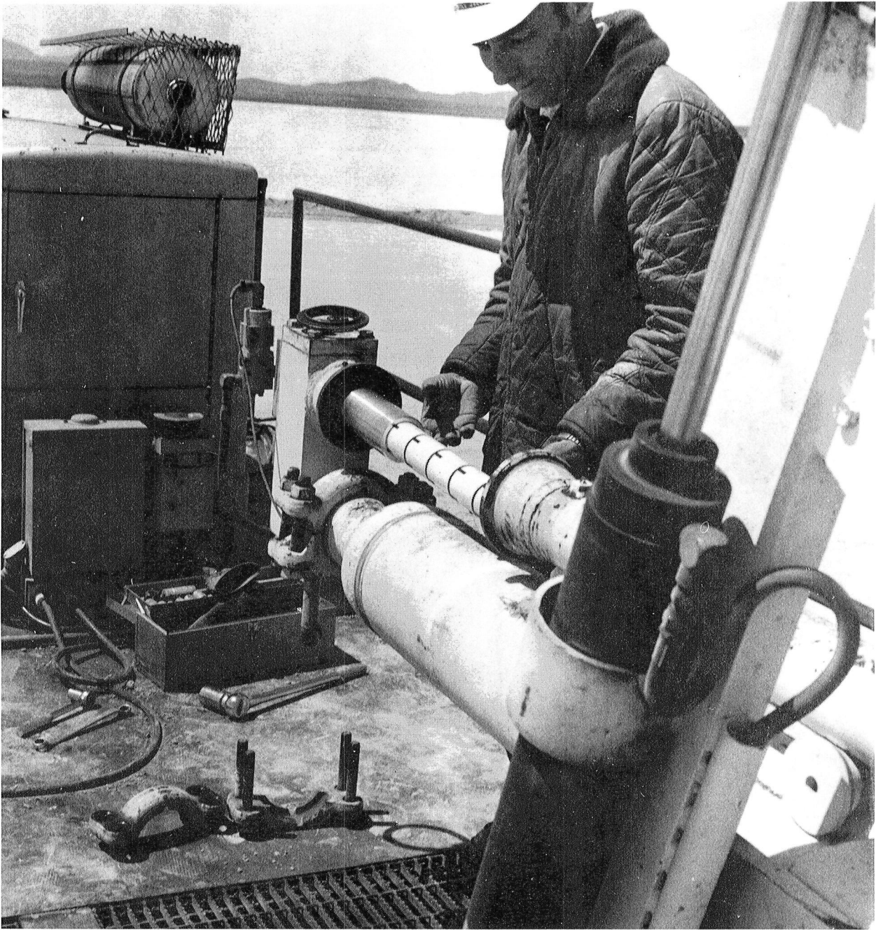
Figure 4.- Penetrator and sabot assembled and mounted in breech of air gun.
