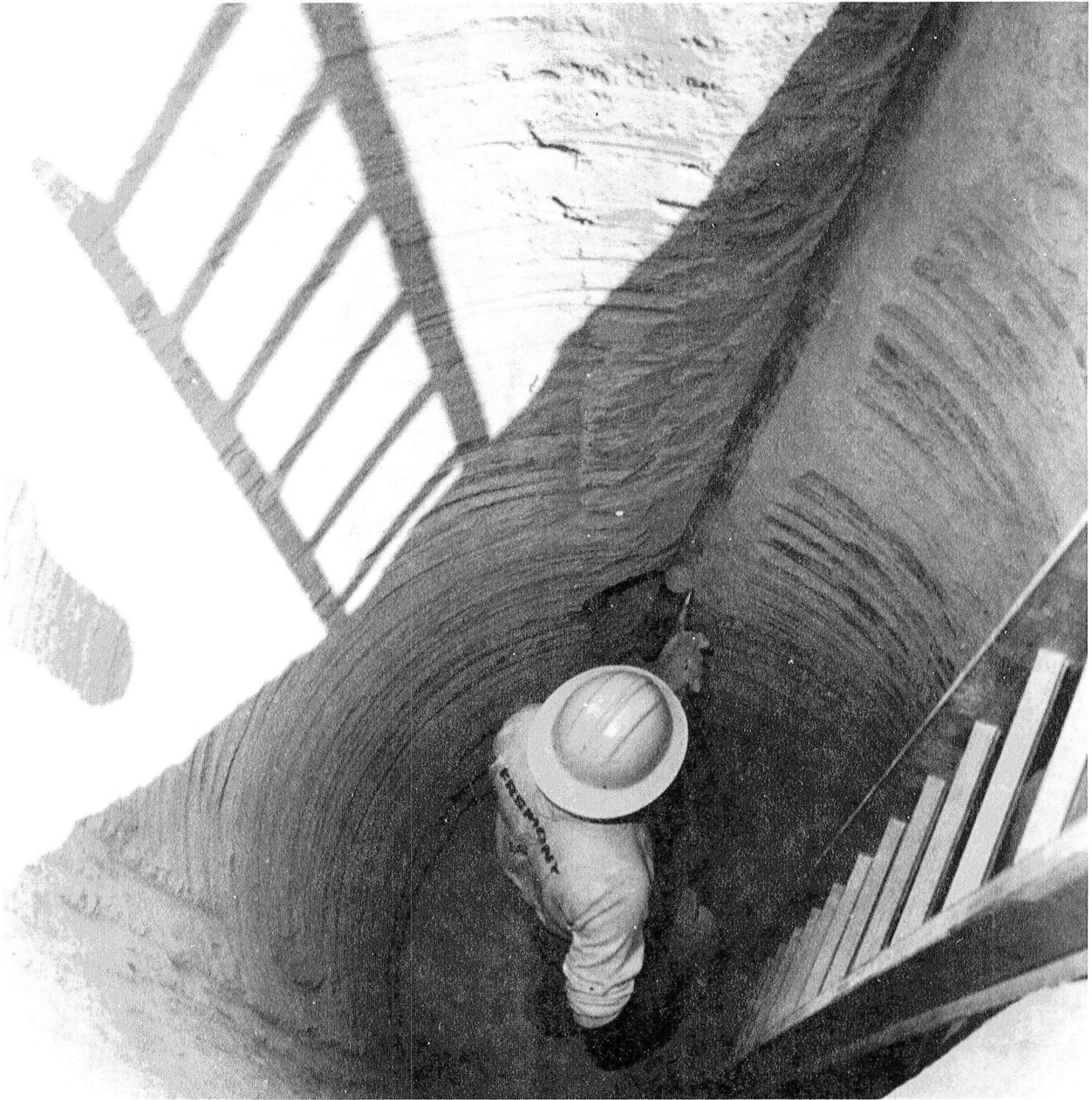
Figure 11.- One side of the hole was removed to expose a complete cross section of the hole made by the penetrator.
