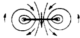
FIG. 33.—Acceleration diagram around an infinitely long flat plate accelerated at right angle to its surface.
