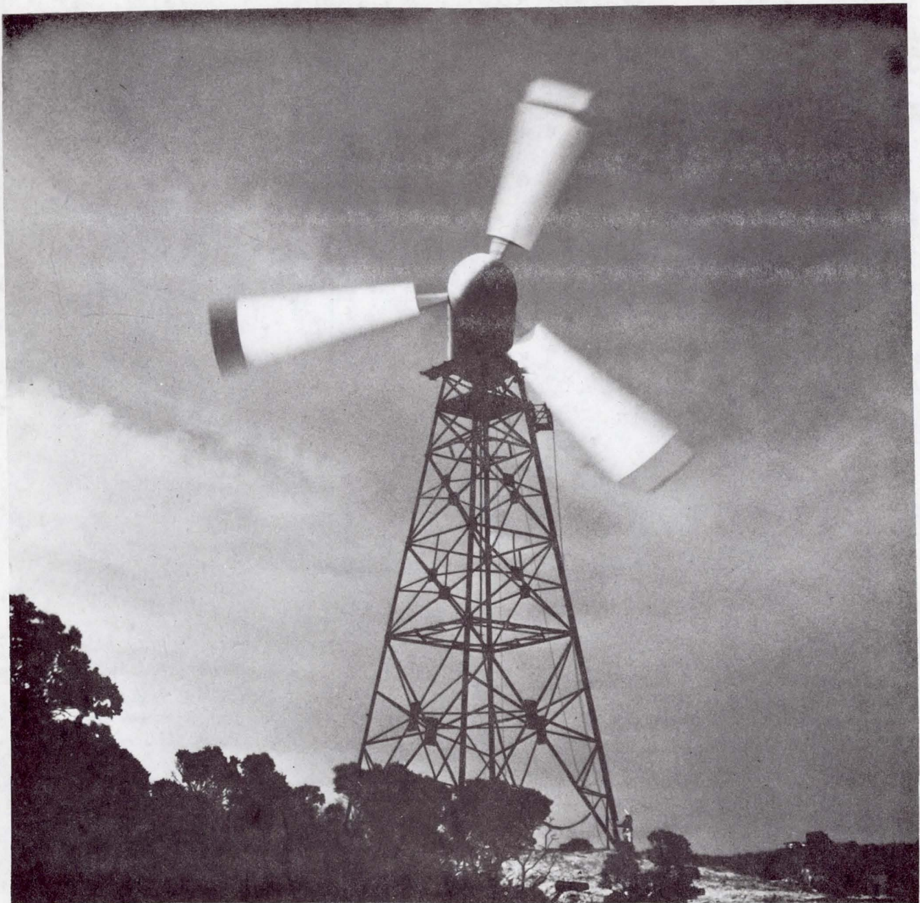
Figure 1. - MP1 - 200 wind turbine generator. (Photo courtesy of Eagle Signal Division, Gulf and Western Manufacturing Company.)
