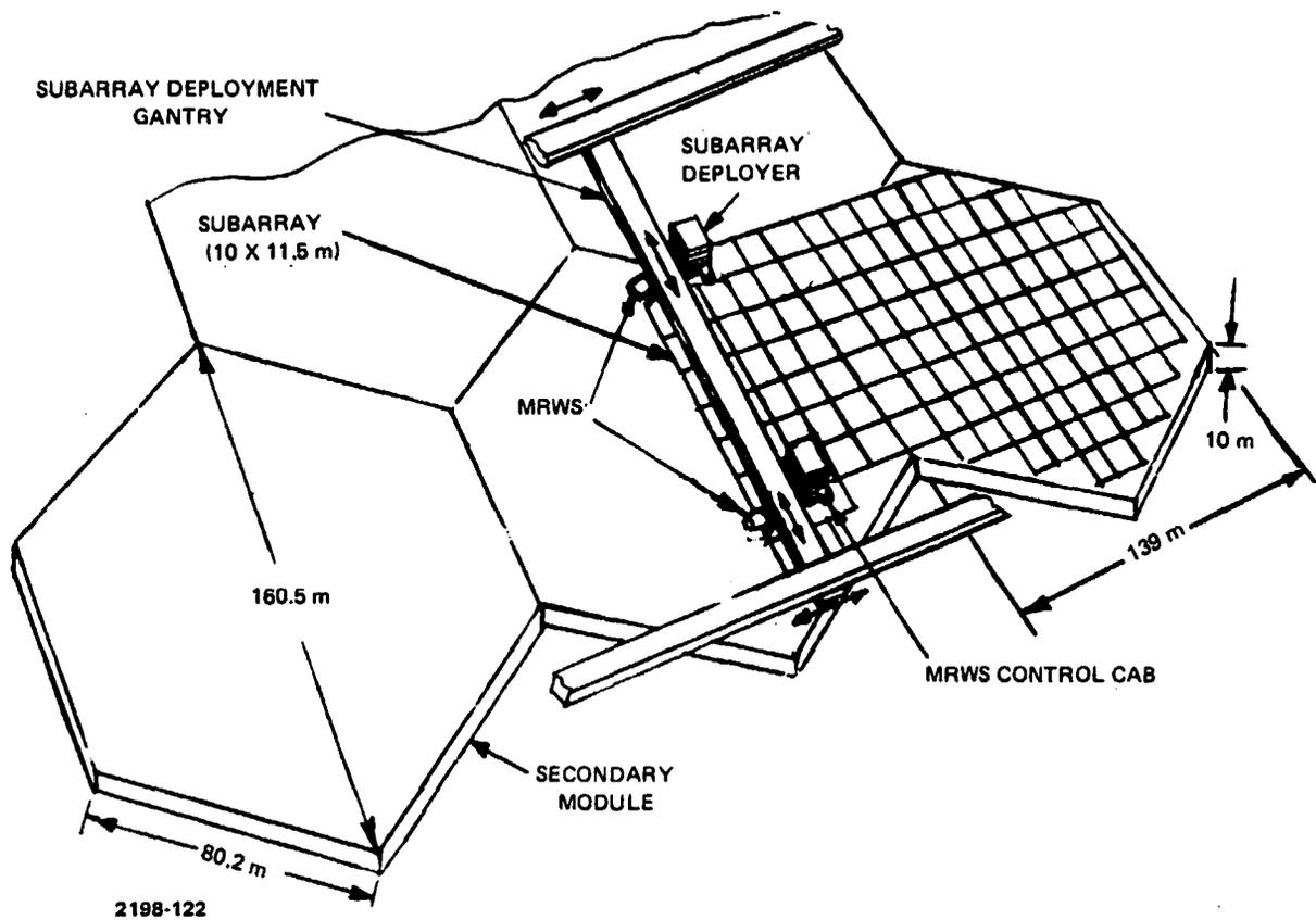
**Figure 107. Microwave Antenna Subarray Installation and Wiring Connections**
