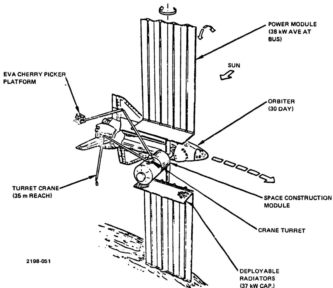
Figure 40. Shuttle Tended Space Construction Base
