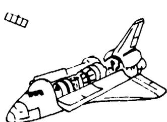
RMS SECURES ST STOWED BY DMP, ORBITER SEPARATES FROM SOLAR ARRAY
