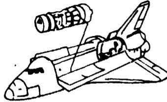
**RMS CAPTURES ST, DMP ROTATED TO BERTHING POSITION**
