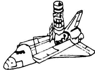
RMS GRAPPLES CAPTURES SOLAR ARRAY. EV CREWMAN DISCONNECTS SOLAR ARRAY FROM ST
