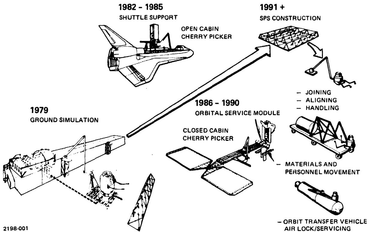
Figure 1. Orbital Construction Support Equipment Development – Universal Manned Remote Work Station
