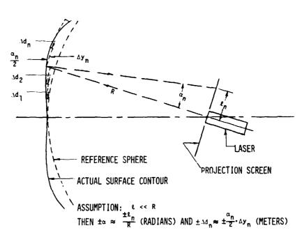
APPROXIMATE SURFACE DEVIATION FROM REFERENCE SPHERE d ≈ 2d1 + 2d2 + ... 2dn
