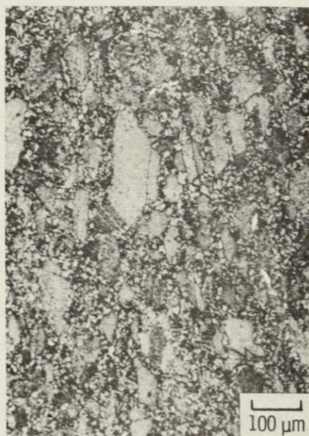
(b) HIP AND FORGED LC ASTROLOY.
