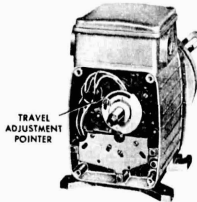
Fig. 4 — Interior view showing travel limit cam on spring return damper actuator.
