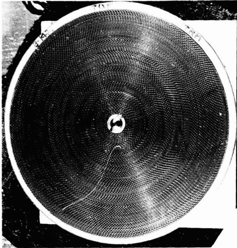
Figure 13-11. Spiral-Wound, Crimped Stainless-Steel Ribbon Core Element, 30.5-cm Diameter by 20.3-cm Length, Posttest Downstream Side
