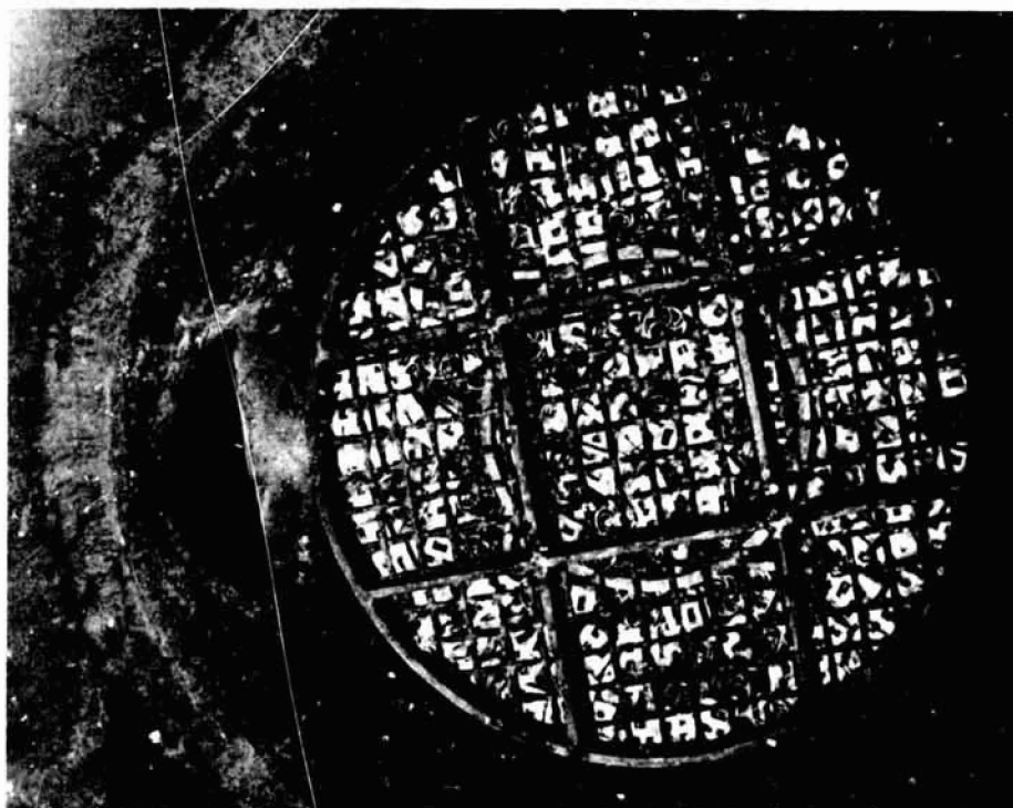
Figure 13-19. Posttest Compacted Bed of Aluminum Ballast Rings
