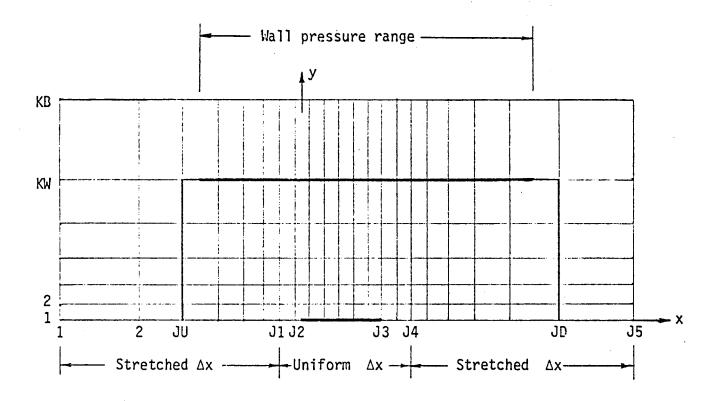
Figure 1.- Schematic representation of upper half of computational grid. Lower half is mirror image about x axis.
